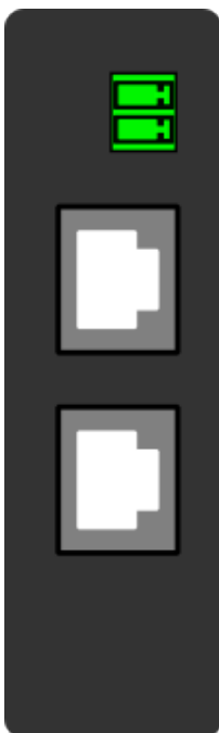
Figure. 8.12 - 262. Double RJ-45 10/100 Mbps Ethernet communication module.
