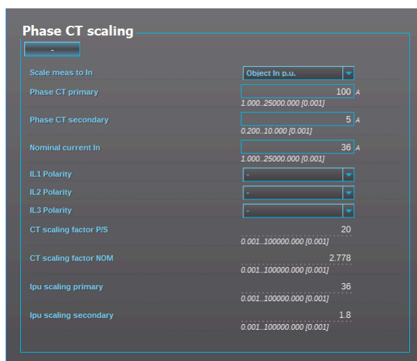
Figure. 5.2.1 - 57. Setting the phase current transformer scalings to the protected object's nominal current.
