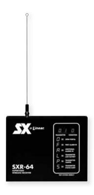
The Model SXR-64A is a 64-channel, 8-zone, supervised wireless receiver/annunciator designed for use in residential or commercial security systems. Housed in a rugged metal enclosure with a high-gain receiver, the SXR-64A connects to a hardwired alarm control panel, adding wireless capability to the panel. The unit's eight alarm zones and four supervisory outputs provide a flexible interface. Any or all of the zones can be used.
