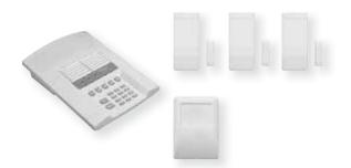
This 12-channel Wireless Security Console Kit contains DVS-1200, three DXS-31 Door/Window Transmitters, one DXS-54 PIR
