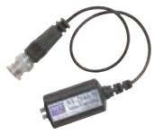
The NVT models NV-208A-M and the NV-214A-M transceivers are passive (non-amplified) devices, which allow the transmission of real-time analog video over unshielded twisted-pair (UTP) telephone wire. "Up-the-Coax" telemetry signals are supported when used with any other passive NVT model including NVT passive hubs.
