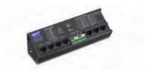
Typically installed in the Wiring Closet or IDF room, the NV-704J-PVD and NV-716J-PVD are passive pass-through wiring devices that efficiently consolidate camera power, video and pan/tilt/zoom data onto a minimum of 4-pair UTP RJ45 cable. Power, video and data are converted at the camera using the NV-218A-PVD or NV-216A-PV transceivers (power and video) which utilize a single 4-pair cable with RJ45 connectors to deliver each camera's signal.
