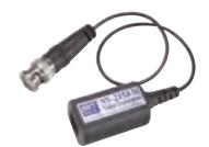
The NVT models NV-215J-M (RJ45) and the NV-217J-M (RJ45) transceivers are passive (non-amplified) devices, which allow the transmission of real-time analog video over unshielded twisted-pair (UTP) telephone wire. "Up-the-Coax" telemetry signals are supported when used with any other passive NVT model including NVT passive hubs.
