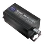
The NVT Model NV-EC1701 Ethernet/PoE over Coax EoC Transceiver is compact media converter that allows 10/100BASE-T Ethernet and PoE power to be transmitted using coax cable. These EoC devices are typically used in legacy installations where existing coax is re-deployed as part of an upgrade to IP cameras. 48 V DC Class 2 power is delivered to one transceiver, which distributes it to up to four remote transceivers and their PoE cameras.
