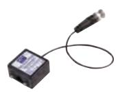
The NVT model NV-218A-PVD Power-Video-Data Transceiver is a passive (non-amplified) device that allows the transmission of real-time monochrome or color video over Category 5e unshielded twisted pair (UTP). Baseband (composite) signals of any type are supported.
