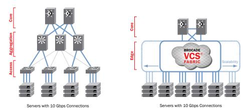
**Figure 1.**Compared to classic Ethernet architectures, Ethernet fabrics allow all paths to be active and provide greater scalability—while reducing management complexity.
