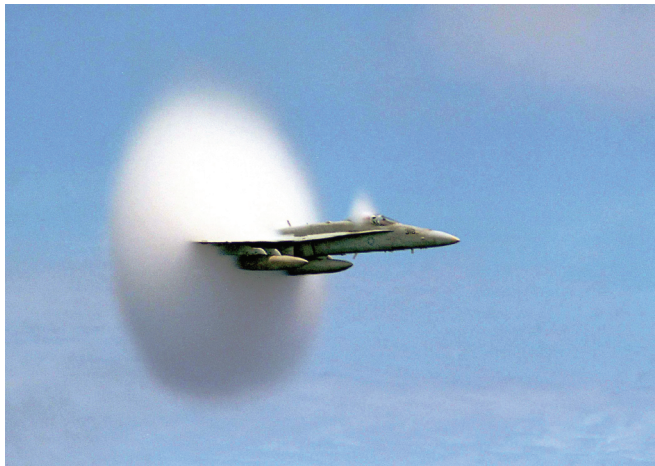
Figure 11. Aerodynamic condensation evidences of supersonic expansion fans around a transonic aircraft.
