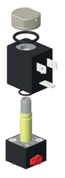
We sell, separately from the coil, a kit to complete the sealing of the 22mm coil, to be equipped on our 22mm pilot valve. The kit is composed by two O-Rings, a special nut designed for this application, and the assembly instruction. Complete valve using coil with terminal has been tested positively for IP65.
