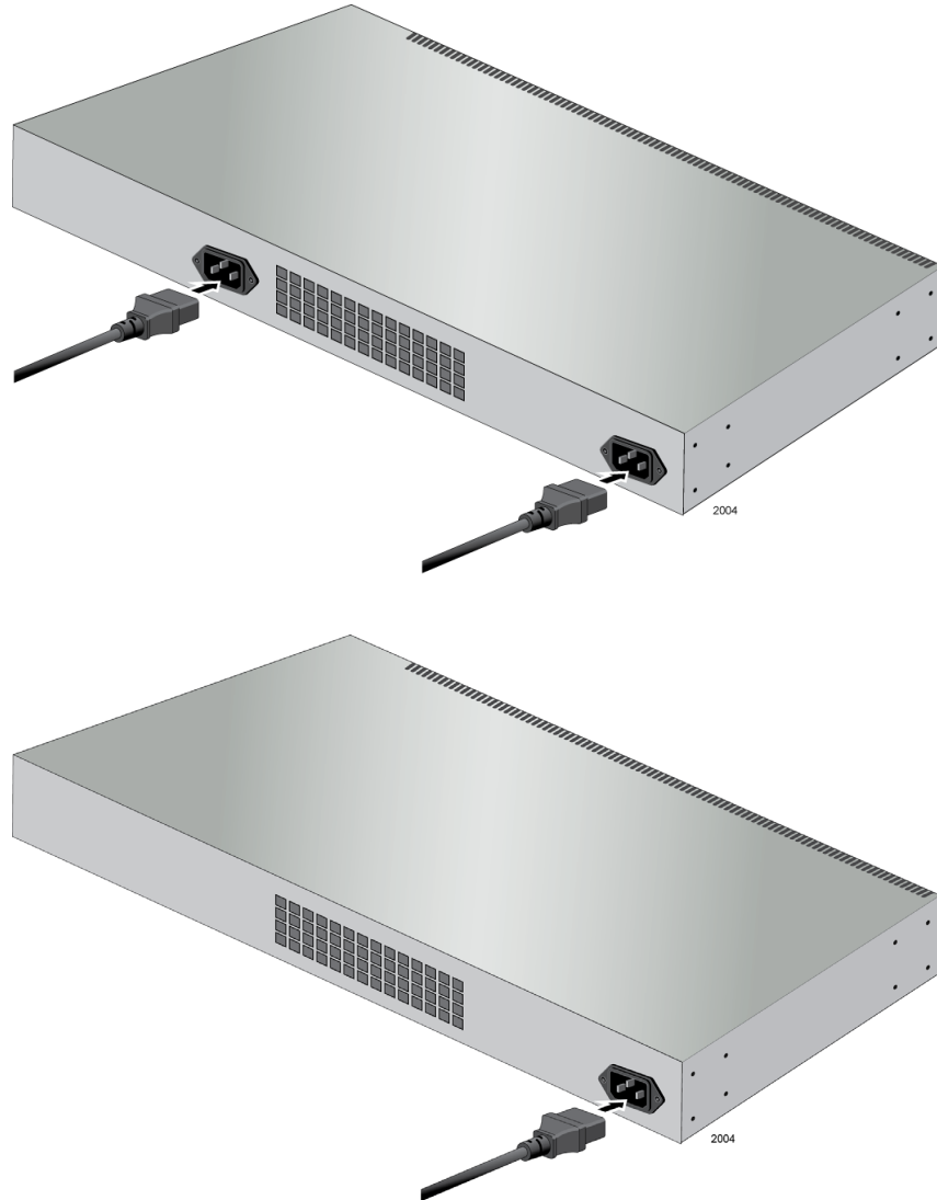
Figure 59. Plugging in the AC Power Cords
