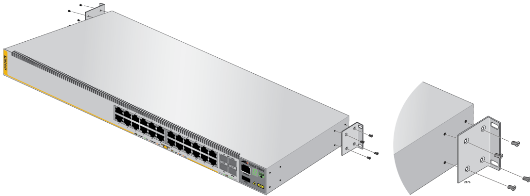
Figure 26. Attaching the Equipment Rack Brackets (Continued)
