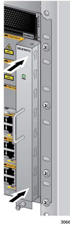
Figure 182. Securing the AT-SBxFAN12 Fan Module on the Backplane Connector
