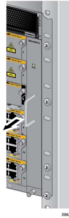
Figure 178. Loosening the AT-SBxFAN12 Fan Module from the Backplane Connector
