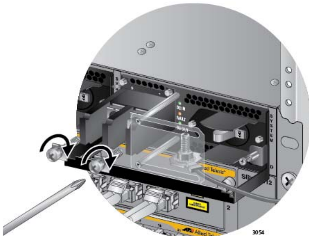
Figure 162. Reinstalling the Screws on the Positive and Negative Terminals
