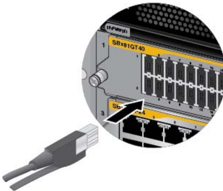
Figure 94. Connecting Cables to Ports on the AT-SBx81GT40 Line Card
