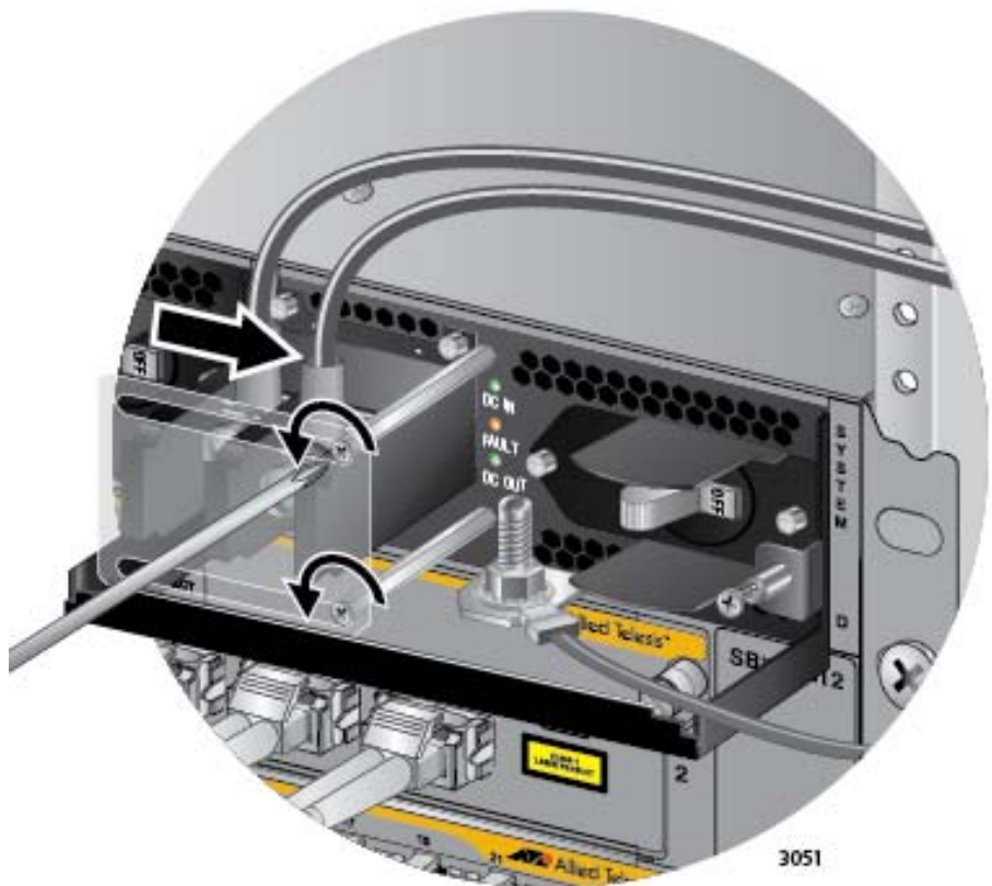
Figure 159. Opening the Plastic Window over the Terminal Block
