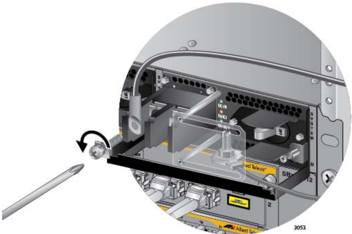
Figure 161. Removing the Positive Lead Wire from the Terminal Block
