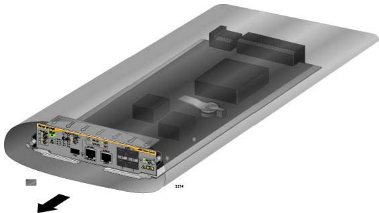
Figure 68. Removing the AT-SBx81CFC960 Controller Fabric Card from the Anti-static Bag
