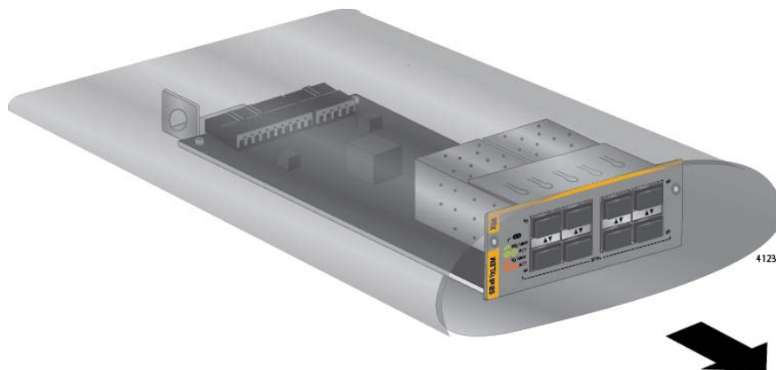
Figure 78. Removing the Expansion Module from the Anti-static Bag
