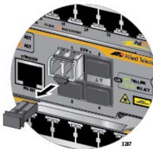
Figure 109. Removing the Dust Cover from an SFP+ Transceiver in the AT-SBx81CFC960 Controller Fabric Card
