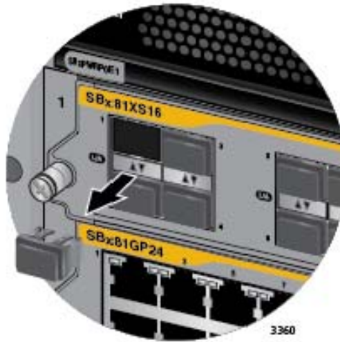
Figure 95. Removing the Dust Cover from a Transceiver Slot
