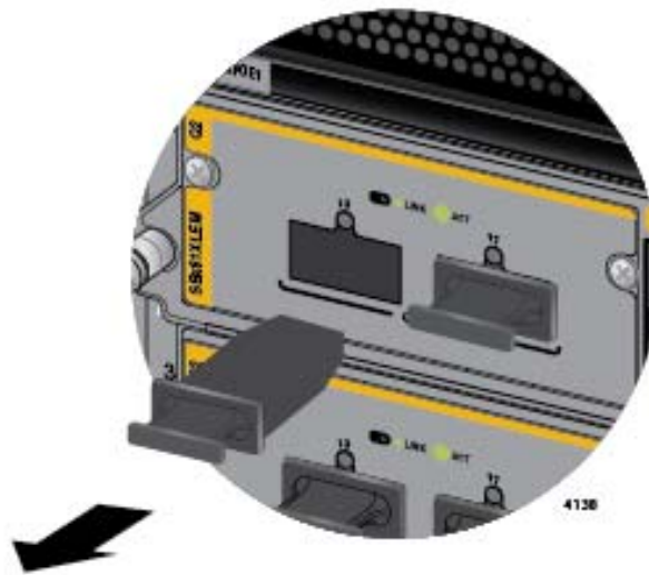
Figure 104. Removing the Dust Cover from a Slot on the AT-SBx81XLEM/Q2 Expansion Module
