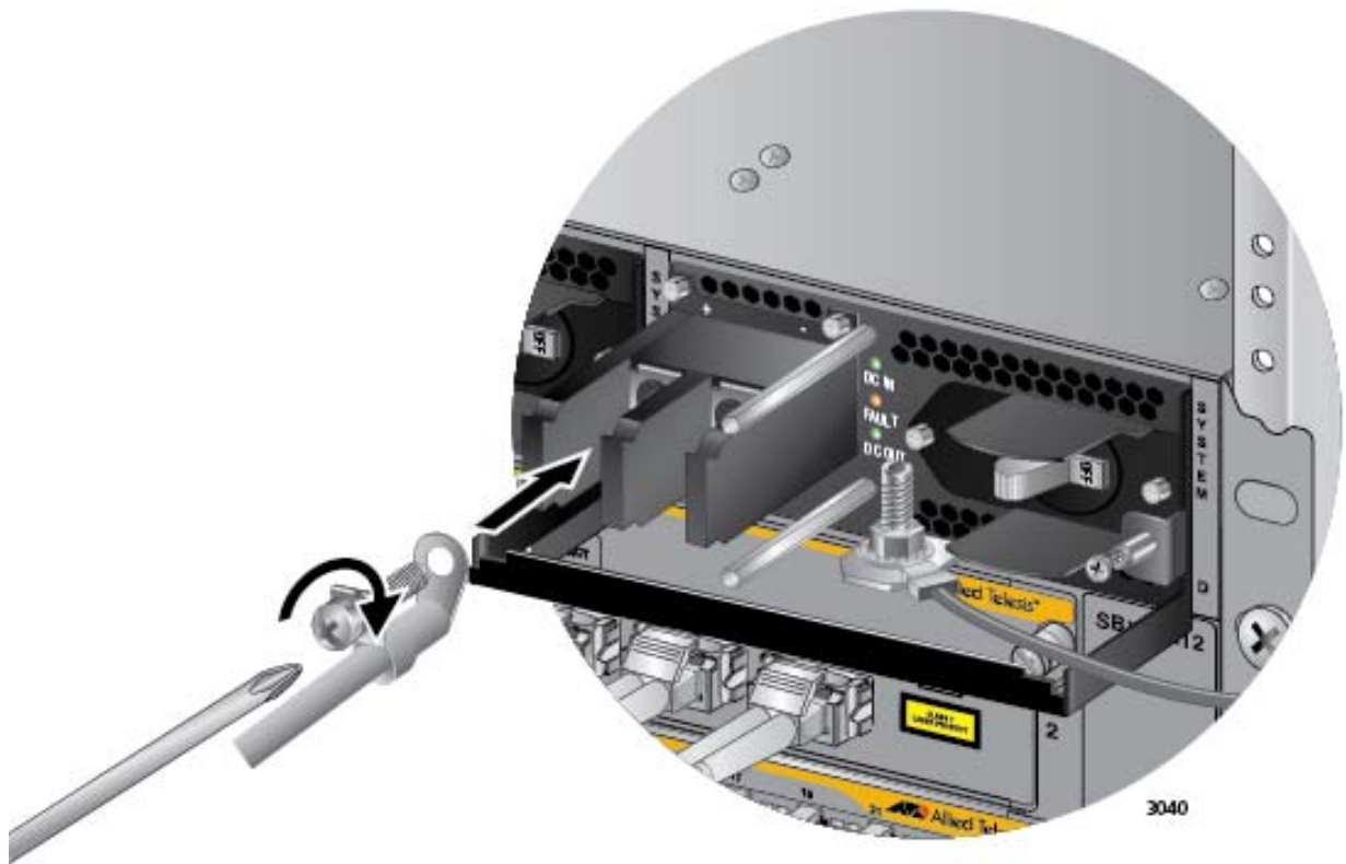
Figure 142. Connecting the Positive (+) Power Wire with a Right Angle Terminal
