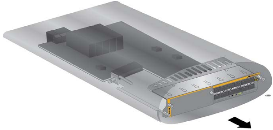
Figure 74. Removing the AT-SBx81XLEM Line Card from the Anti-static Bag
