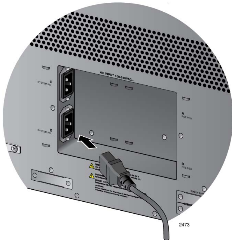
Figure 114. Connecting the AC Power Cord for the AT-SBxPWRSYS1 or AT-SBxPWRSYS2 AC System Power Supply
