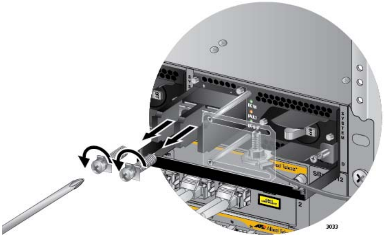
Figure 133. Removing the Terminal Screws
