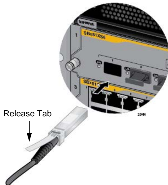
Figure 103. Installing the AT-SP10TW Cable in the AT-SBx81XS6 Line Card
