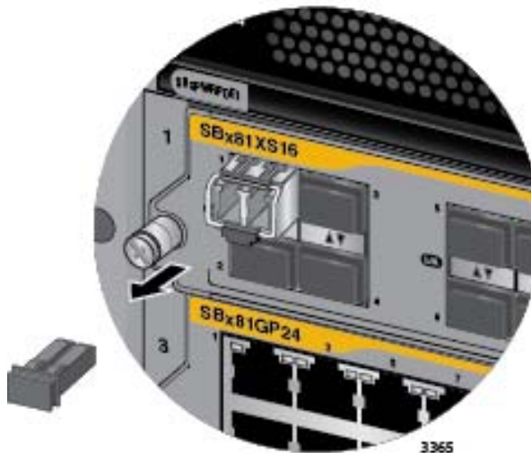
Figure 98. Removing the Dust Cover from a Transceiver
