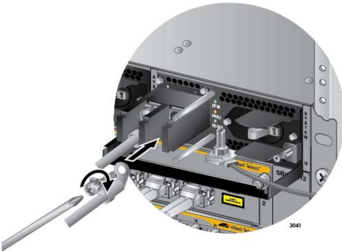
Figure 143. Connecting the Negative (-) Power Wire with a Right Angle Terminal
