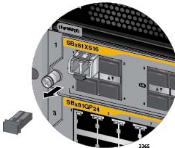
Figure 93. Removing the Dust Cover from a Transceiver in the AT-SBx81XS16 Line Card
