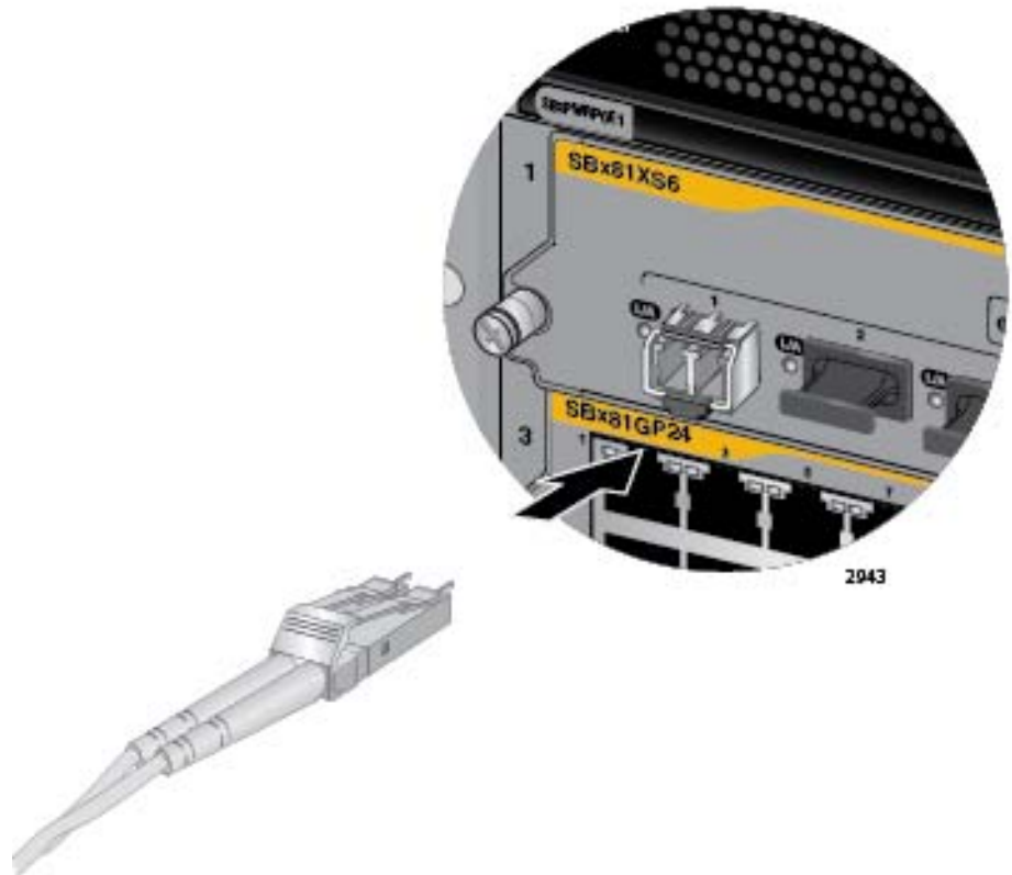
Figure 88. Attaching a Fiber Optic Cable to an SFP+ Transceiver in the AT-SBx81XS6 Line Card
