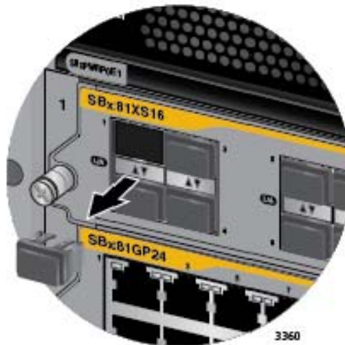
Figure 91. Removing the Dust Cover from a Transceiver Slot in the AT-SBx81XS16 Line Card
