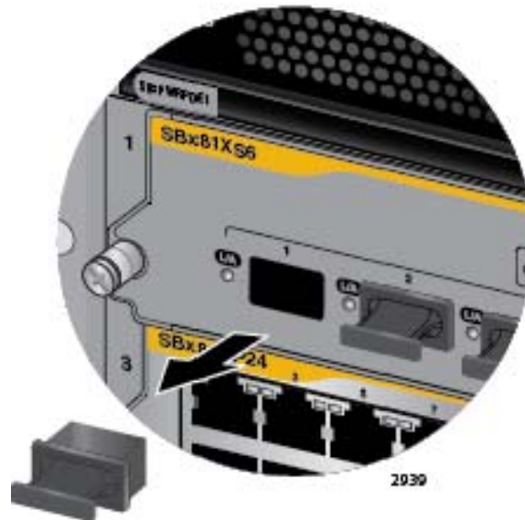
Figure 83. Removing the Dust Cover from an SFP+ Slot in the AT-SBx81XS6 Line Card
