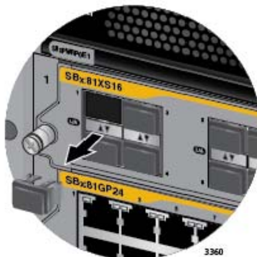
Figure 96. Removing the Dust Cover From an SFP+ Slot on the AT-SBx81XS16 Line Card
