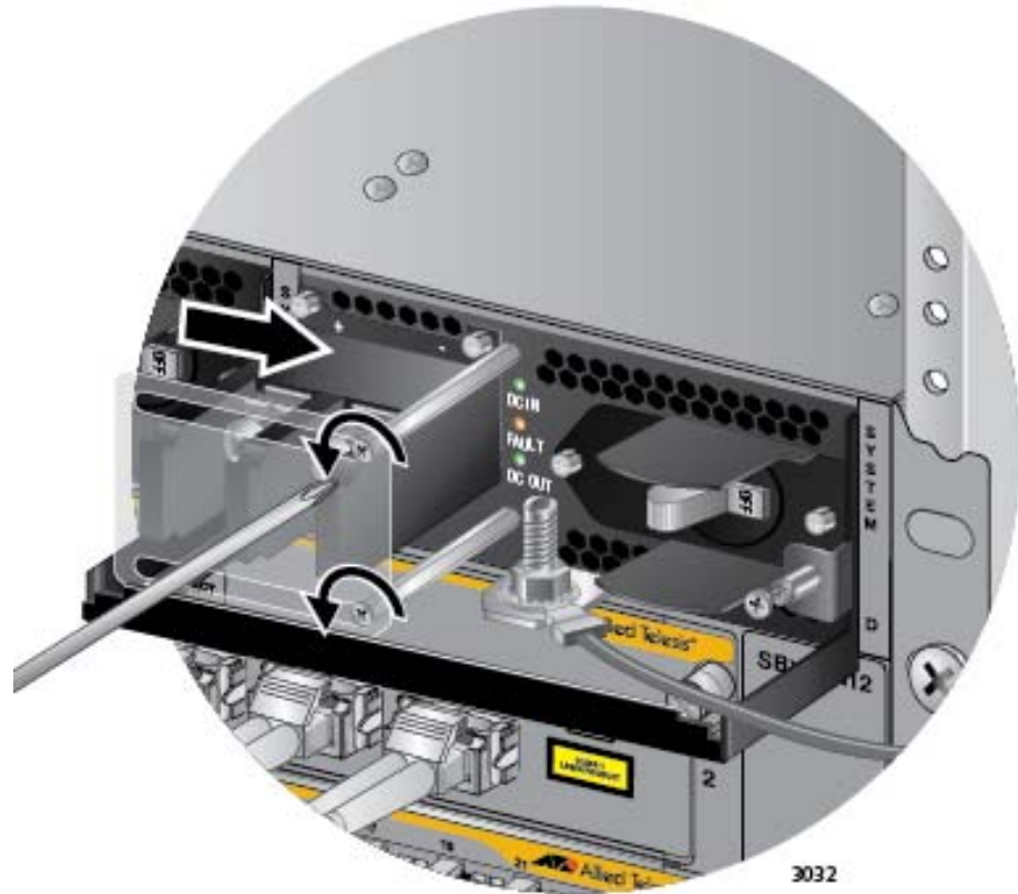
Figure 124. Opening the Plastic Cover
