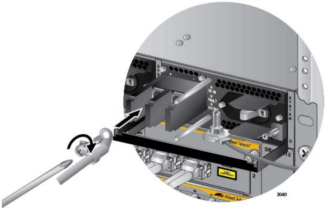
Figure 134. Connecting the Positive (+) Power Wire with a Right Angle Terminal
