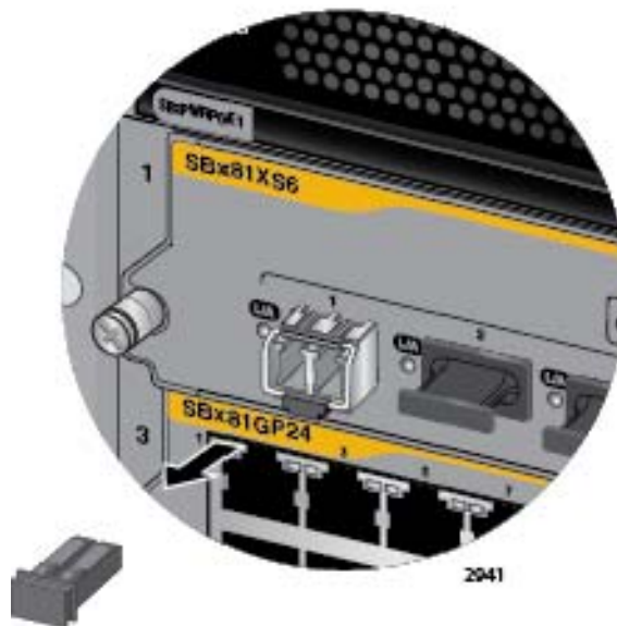
Figure 86. Removing the Dust Cover from an SFP+ Transceiver in the AT-SBx81XS6 Line Card
