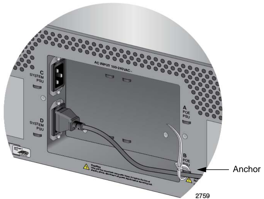
Figure 117. Securing the Power Cord for the AT-SBxPWRSYS1 or AT-SBxPWRSYS2 AC System Power Supply to an Anchor
