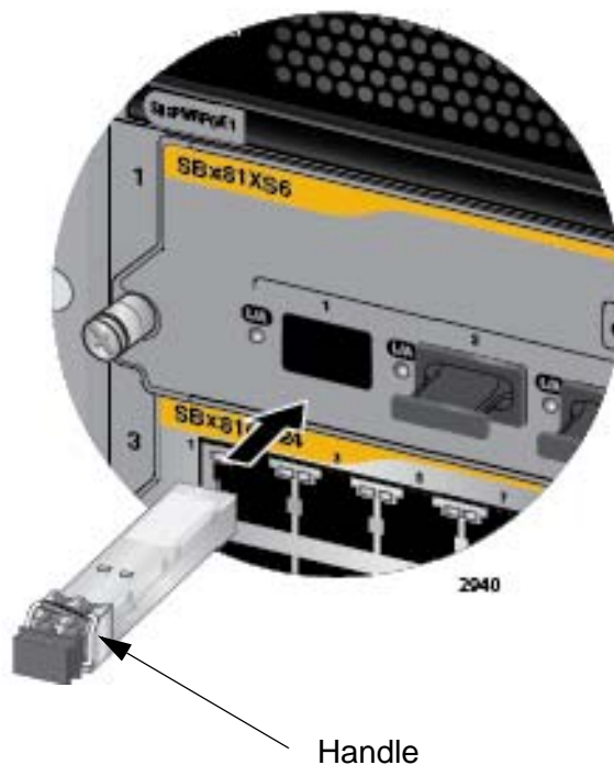
Figure 99. Installing an SFP+ Transceiver in the AT-SBx81XS6 Line Card
