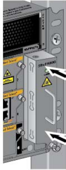
Figure 184. Securing the AT-SBxFAN06 Fan Module on the Backplane Connector
