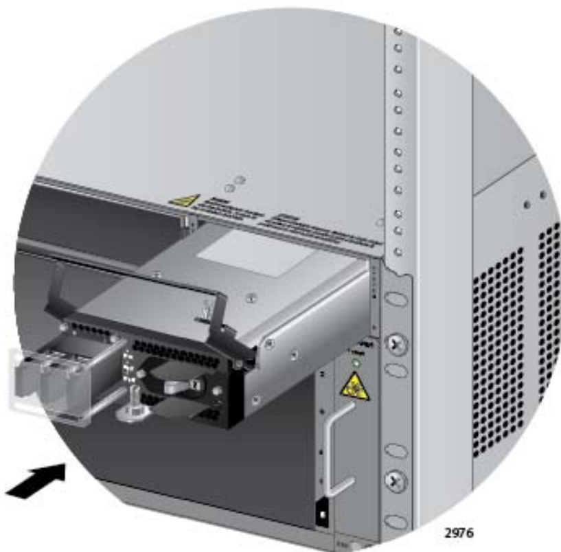
Figure 66. Inserting the AT-SBxPWRSYS1 DC System Power Supply
