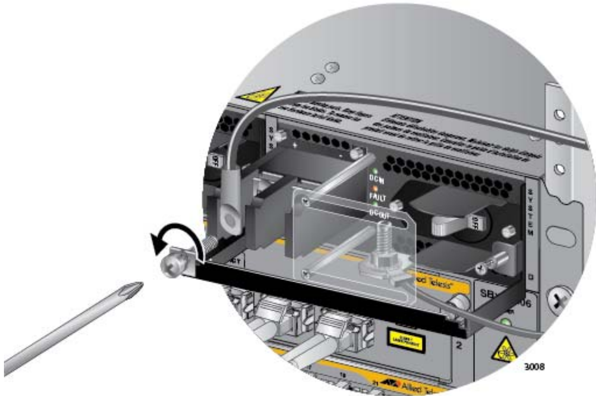
Figure 163. Removing the Positive Lead Wire from the Terminal Block
