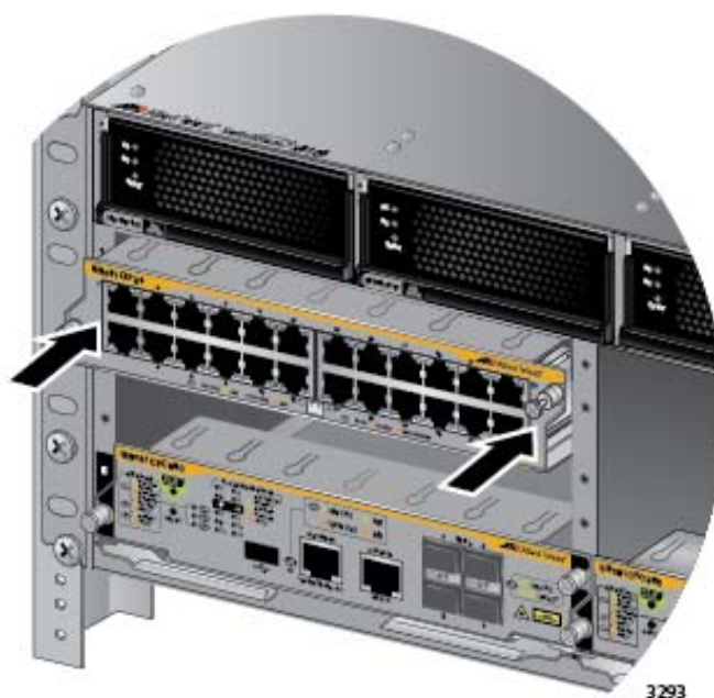
Figure 91. Seating an Ethernet Line Card on the Backplane Connector
