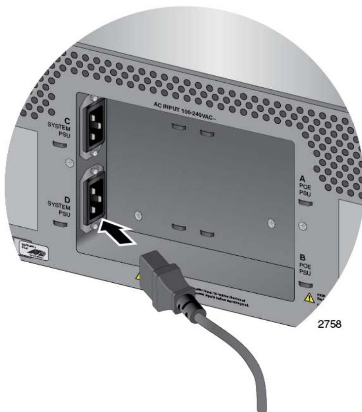
Figure 116. Connecting the AC Power Cord for the AT-SBxPWRSYS1 or AT-SBxPWRSYS2 AC System Power Supply
