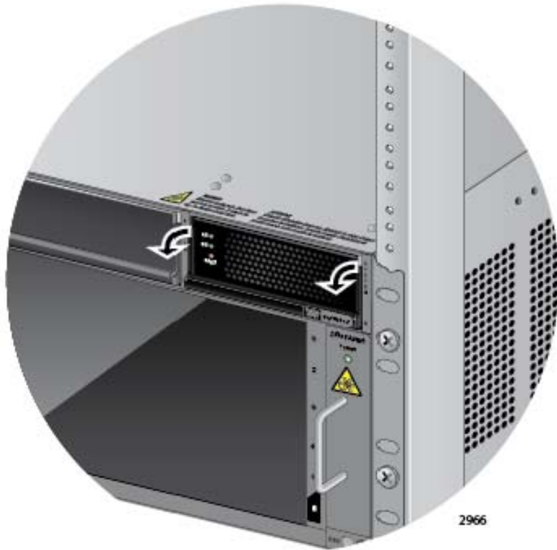
Figure 55. Lowering the Handle on the AT-SBxPWRSYS1 or AT-SBxPWRSYS2 AC System Power Supply
