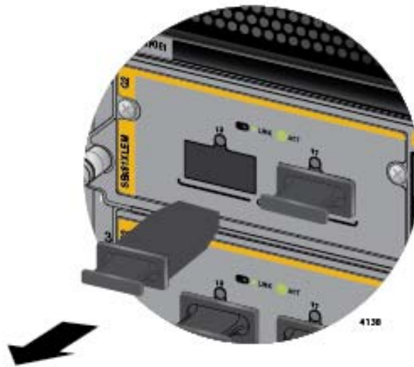
Figure 106. Removing the Dust Cover from a Slot on the AT-SBx81XLEM/Q2 Expansion Module
