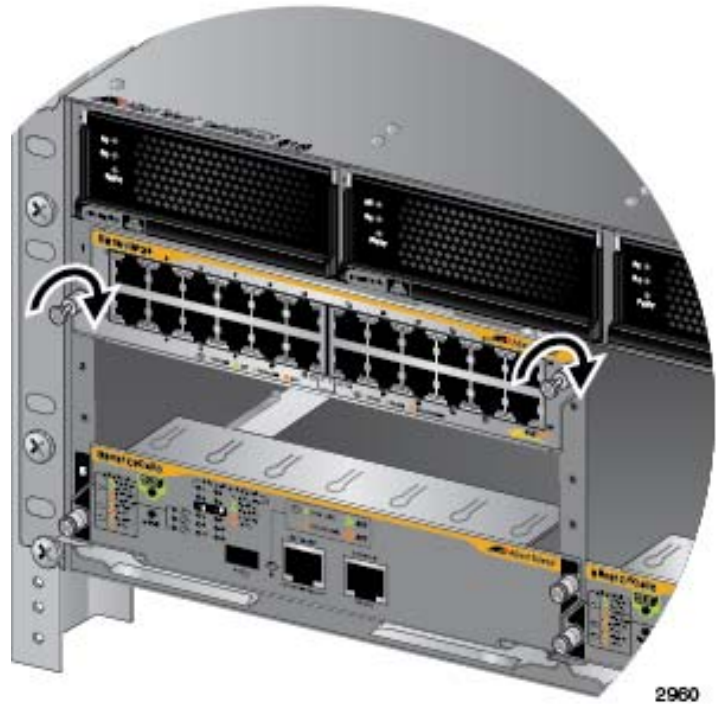
Figure 72. Tightening the Thumb Screws on an Ethernet Line Card
