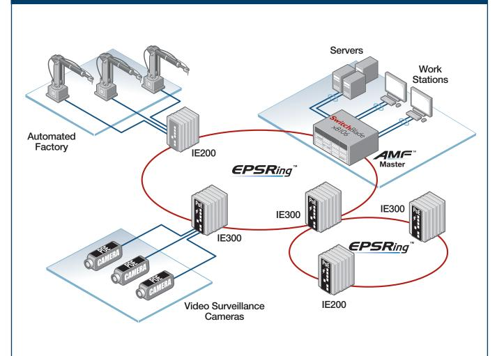
Ethernet Protection Switched Ring (EPSRing<sup>™</sup>) and ITU-T G.8032 provide high speed resilient ring connectivity; this diagram shows the IE Series in a double ring network topology.
