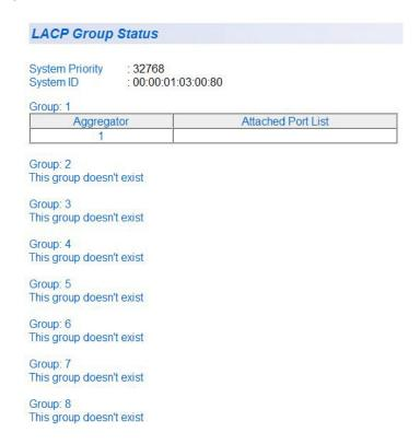
Figure 33. LACP Group Status Page with No Cables Connected
