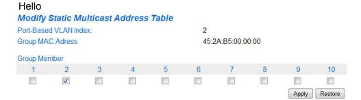
Figure 43. Modify Static Multicast Address Page
