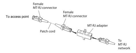
Figure 18. Connecting to an MT-RJ Network
