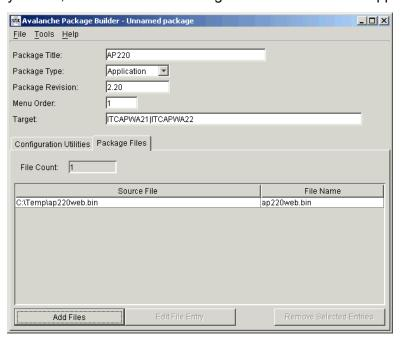
2. Create a software package (.AVA file) that includes the latest software release (.BIN file) using Avalanche Package Builder.
