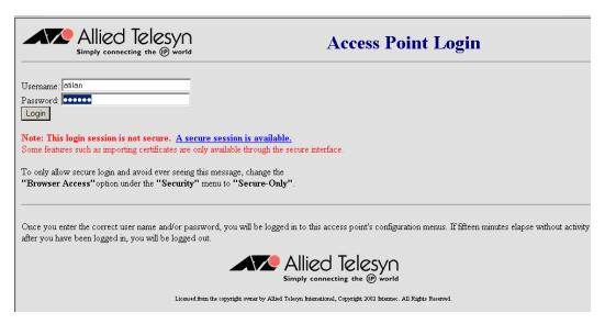
4. If necessary, enter a user name and a password. The default user name is "atilan" and the default password is "atilan". You can define a user name and password. For help, see "Setting Up Logins" on page 176.
