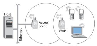
Figure 11. 802.11g WAP with No Roaming End Devices
