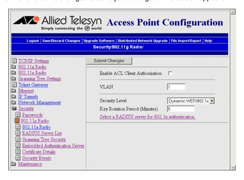
In the Key Rotation Period (Minutes) field, enter how often (in minutes) the access point generates a new WEP key to distribute to the end devices.
