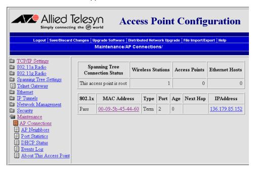
2. Click an IP address hyperlink. The access point pings the device, and then the Ping Utility screen appears showing the results.
