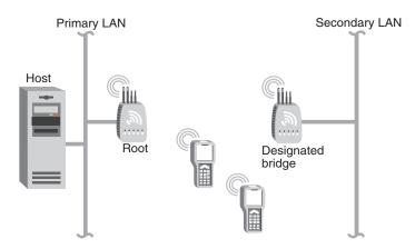
Figure 15. 802.11a Point-to-Point Bridges
