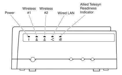
Figure 2. AT-WA7501 LEDs
