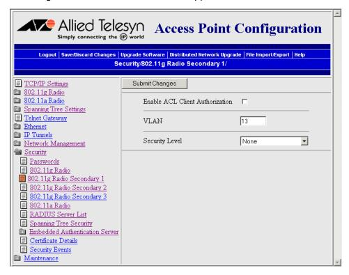
6. In the VLAN field, enter the VLAN number that encapsulates all frames received on this radio port. This value must match the values that are set in the VLAN-capable Ethernet switches on the primary LAN.
