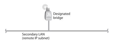
Within the spanning tree, access points use IAPP (Inter Access Point Protocol) or secure IAPP to communicate with each other across the Ethernet network, over wireless secondary LANs, and through IP tunnels to remote IP subnets. IAPP also enables fast roaming in an 802.11g, 802.11b or 802.11a network using 802.1x security. Secure IAPP prevents unauthorized access products from joining the spanning tree.
