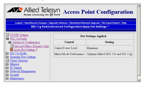
Configuring the 802.11g Radio to Communicate With a SpectraLink Network
