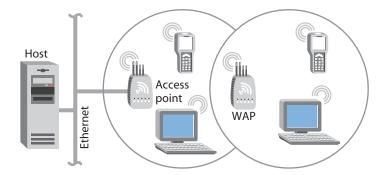
Figure 12. 802.11a WAP with Roaming End Devices
