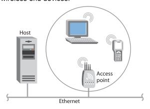
Figure 6. Simple Wireless Network
