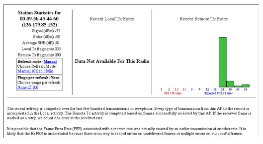
By default, the Refresh Mode is Manual. To configure the software to refresh automatically at a set interval, click 10 Sec or 1 Min.
