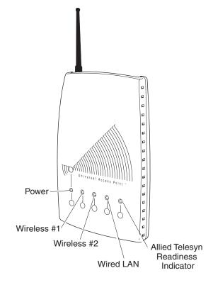
Figure 3. AT-WA7500 LEDs
