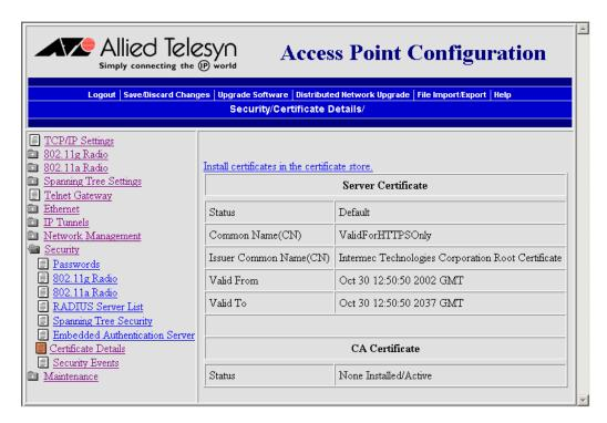
The Server Certificate table lists the server certificate that is installed, and the CA Certificate table lists the trusted CA certificate that is installed.
