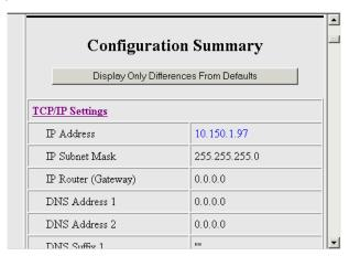
Click the button under the Configuration Summary title to switch between displaying all configuration settings and displaying the configuration settings that are different from the factory default settings.
