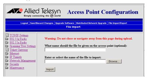
2. (Optional) You can type a filename in the first input field to specify the name that the file will have on the access point.
