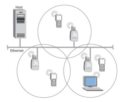
Figure 8. Multiple Access Points with Roaming End Devices
