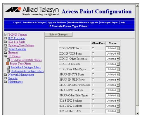
2. For each frame type field, check or clear the check box to configure if the frame types are passed or are dropped. If you check the check box, the frame type is allowed to pass.
