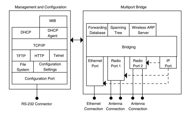
Figure 1. Access Point Architecture
