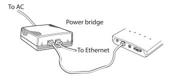
Figure 19. Power Over Ethernet
