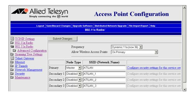
b. Make sure the Allow Wireless Access Points field is On Primary.
