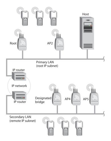
IP tunnels use encapsulation to establish a virtual LAN (VLAN) segment through IP routers. The VLAN segment includes the root IP subnet and logically extends to include end devices attached to access points on remote IP subnets. IP tunnels are branches in the spanning tree topology.
