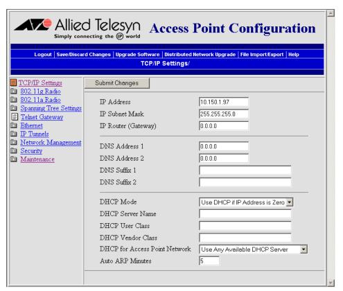
2. Configure the DHCP parameters to make this access point a DHCP client. For help, see the next table.
