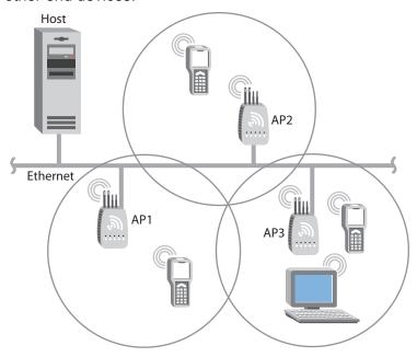
Figure 9. 802.11g Access Point with Roaming End Devices
