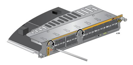
Figure 80. Securing the Expansion Module
