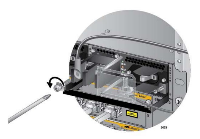
Figure 153. Removing the Positive Lead Wire from the Terminal Block
