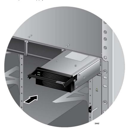
Figure 50. Inserting the AT-SBxPWRSYS1 or AT-SBxPWRSYS2 AC System Power Supply
