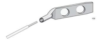
Figure 43. Attaching the Grounding Wire to the Grounding Lug
