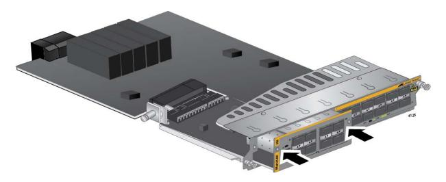
Figure 79. Seating the Expansion Module on the Connector in the AT-SBx81XLEM Line Card
