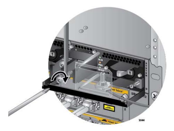
Figure 139. Connecting the Negative Lead Wire with Bare Wire
