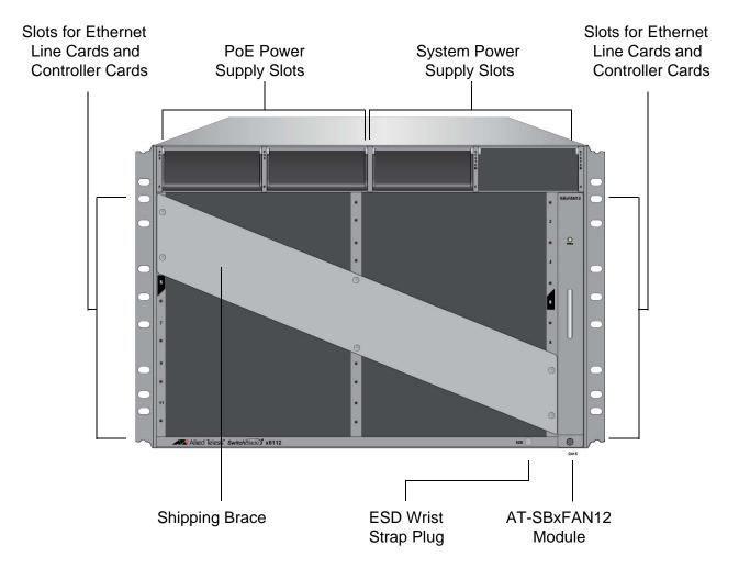
Figure 2. Front View of the AT-SBx8112 Chassis
