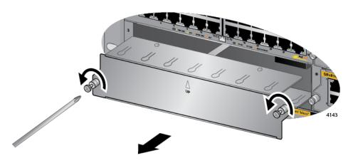
Figure 85. Removing a Blank Slot Cover
