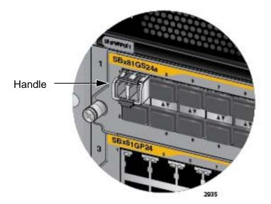
Figure 98. Verifying the Position of the Handle on a Transceiver
