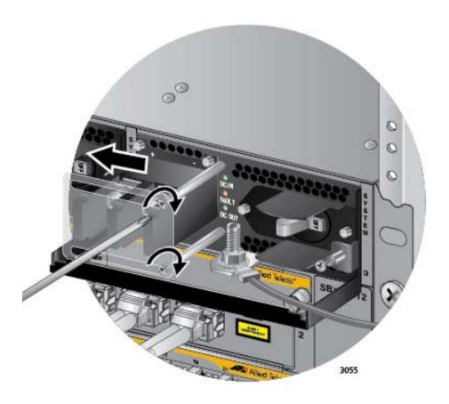
Figure 155. Closing the Plastic Cover
