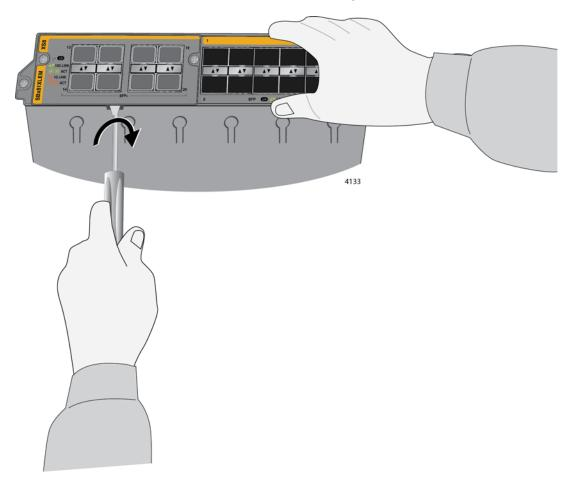
Figure 163. Disconnecting the Expansion Module from the AT-SBx81XLEM Line Card
