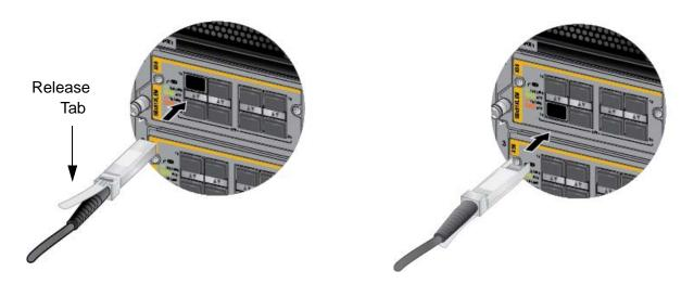
Figure 102. Installing the AT-SP10TW Cable in the AT-SBx81XLEM/XS8 Expansion Module
