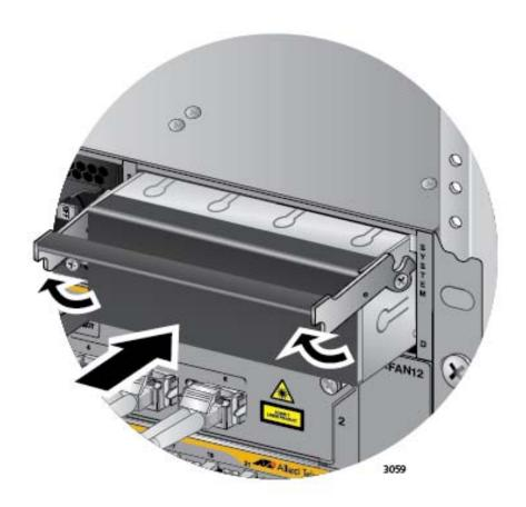
Figure 159. Installing a Blank Power Supply Slot Cover
