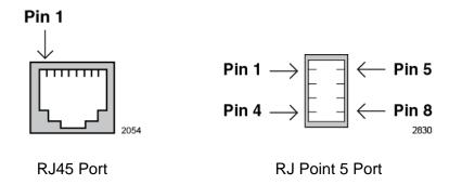
Figure 176. Pin Numbers for RJ-45 and RJ Point 5 Ports (Front View)
