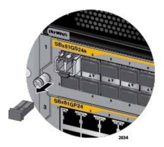
Figure 97. Removing the Dust Cover from a Transceiver
