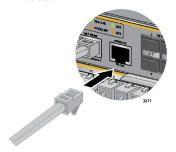
Figure 142. Connecting the Management Cable to the Console RS-232
