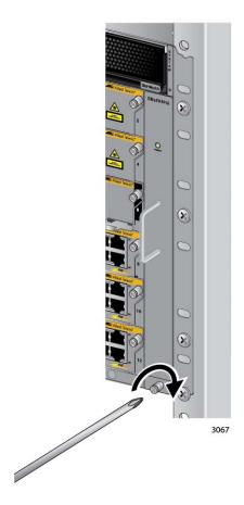
Figure 175. Tightening the Screw on the AT-SBxFAN12 Fan Module
