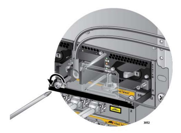
Figure 152. Removing the Negative Lead Wire
