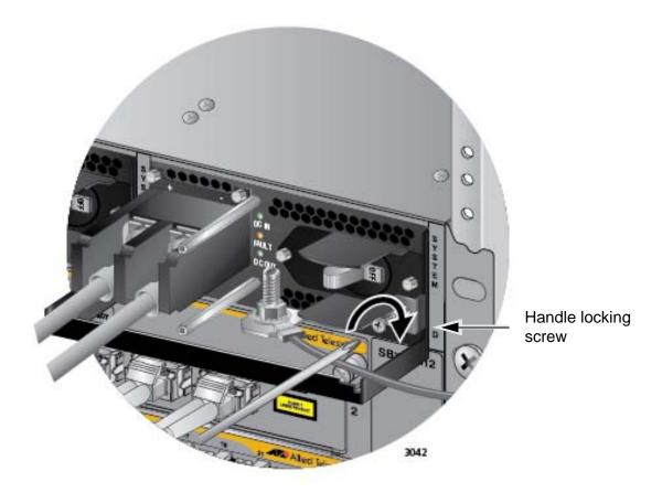
Figure 136. Tightening the Handle Locking Screw
