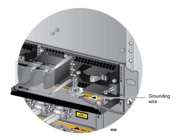
Figure 116. Installing the Grounding Wire
