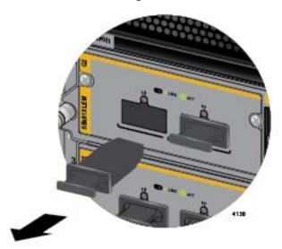
Figure 103. Removing the Dust Cover from a Slot on the AT-SBx81XLEM/
