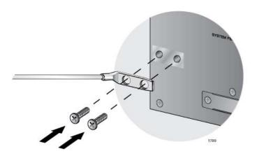
Figure 44. Installing the Grounding Lug and Wire
