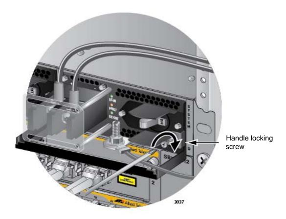
Figure 129. Tightening the Handle Locking Screw
