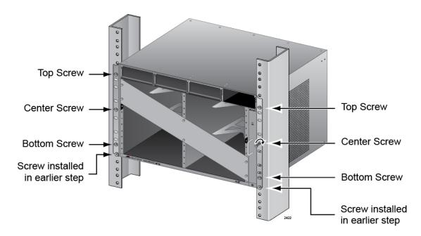
Figure 39. Installing the Rack Mount Screws
