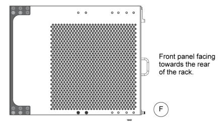
Figure 37. Rack Bracket Locations for Reverse Position of Chassis
