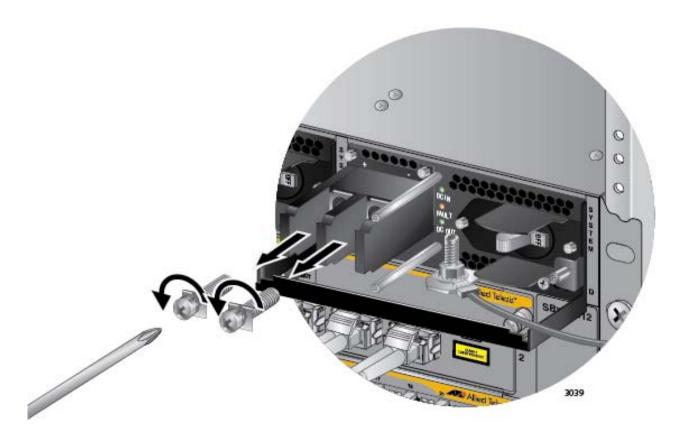
Figure 133. Removing the Terminal Screws
