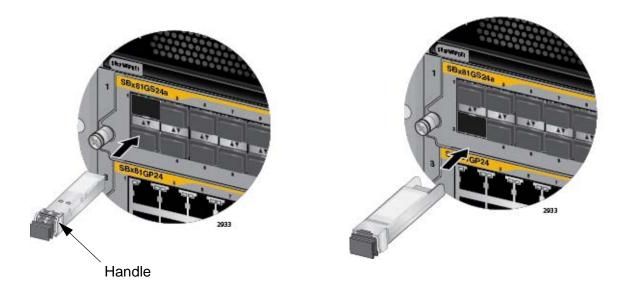
Figure 95. Inserting an SFP or SFP+ Transceiver
