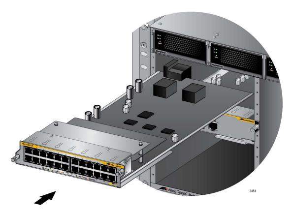
Figure 87. Aligning an Ethernet Line Card in a Chassis Slot
