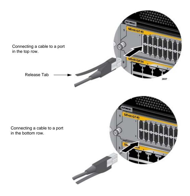
Figure 93. Connecting Cables to Ports on the AT-SBx81GT40 Line Card
