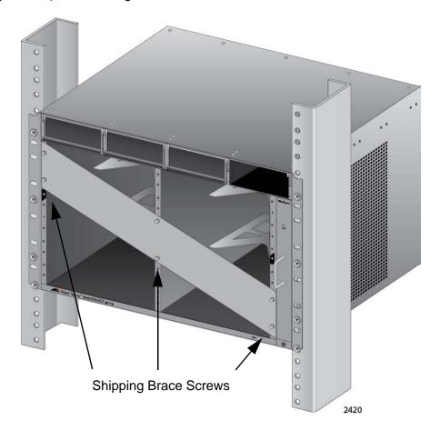
Figure 40. Removing the Shipping Brace
