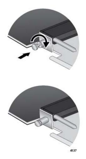
Figure 168. Releasing the Retaining Pin
