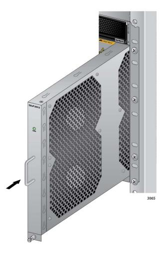
Figure 173. Installing a New AT-SBxFAN12 Fan Module
