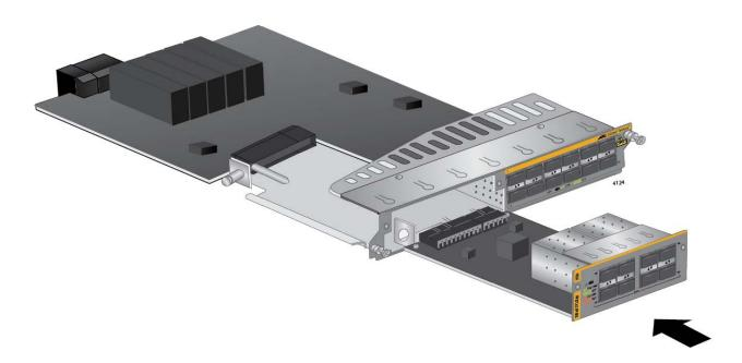
Figure 78. Sliding the Expansion Module into the AT-SBx81XLEM Line Card
