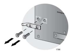
Figure 42. Removing the Grounding Lug
