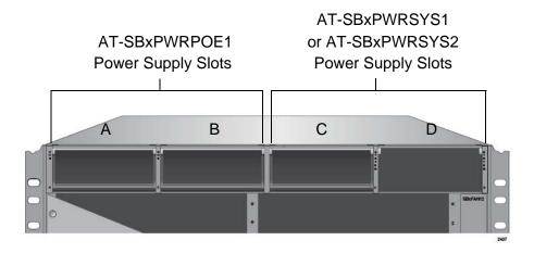
Figure 46. Power Supply Slots
