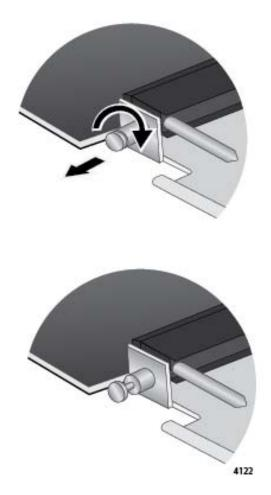
Figure 76. Retracting the Retaining Pin on the AT-SBx81XLEM Line Card
