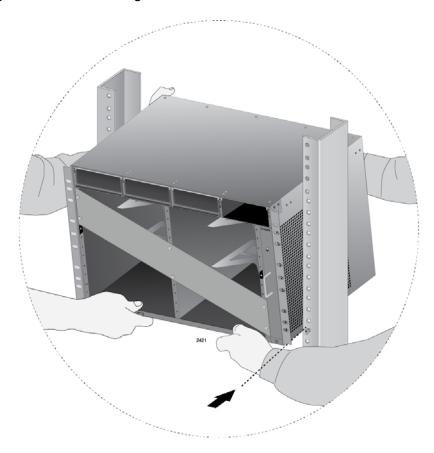
Figure 38. Lifting the AT-SBx8112 Chassis into the Equipment Rack
