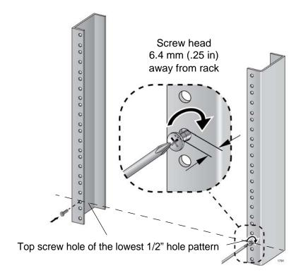
Figure 33. Rack Mounting Hole Locations
