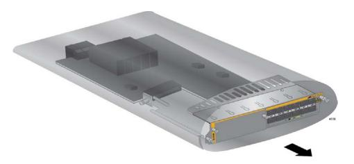
Figure 73. Removing the AT-SBx81XLEM Line Card from the Anti-static Bag
