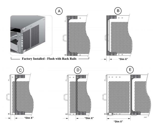
Figure 36. Rack Mounting Bracket Locations
