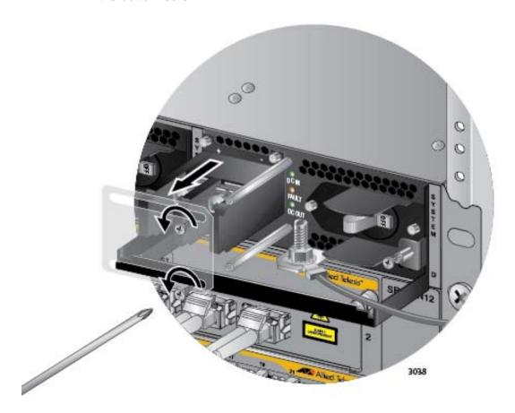
Figure 132. Removing the Plastic Cover
