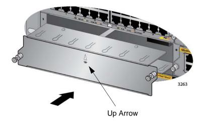
Figure 90. Installing a Blank Slot Cover
