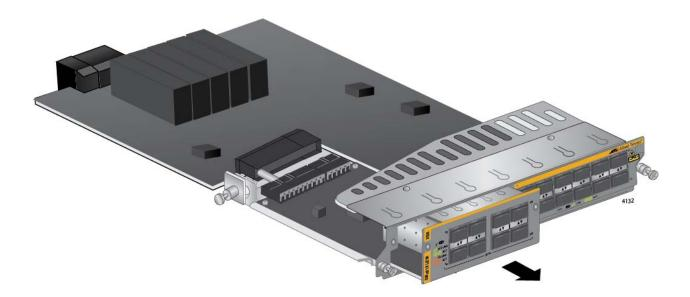
Figure 164. Sliding the Expansion Module from the AT-SBx81XLEM Line Card
