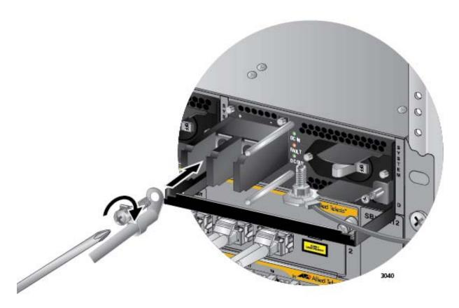
Figure 134. Connecting the Positive (+) Power Wire with a Right Angle Terminal
