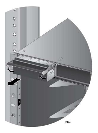
Figure 52. Removing the Blank Slot Cover from Power Supply Slot A
