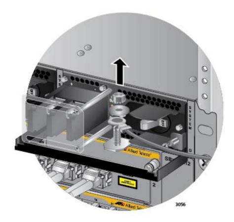
Figure 156. Removing the Grounding Wire
