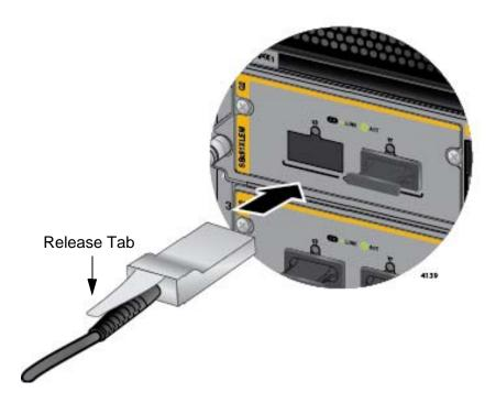
Figure 104. Sliding the AT-QSFPCU Cable into the Slot
