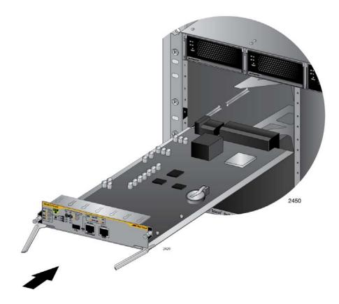
Figure 70. Aligning the AT-SBx81CF400 Card in the Chassis Slot
