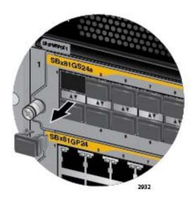
Figure 94. Removing the Dust Cover from an SFP or SFP+ Slot
