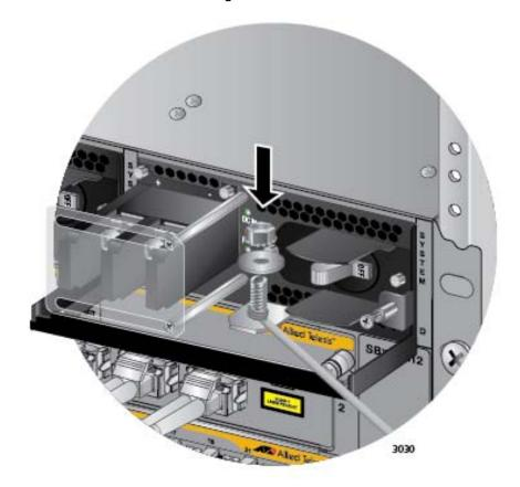
Figure 119. Securing the Bare Grounding Wire to the Grounding Post Allied Telesis recommends tightening the nut and washer to 26 inchlbs.
