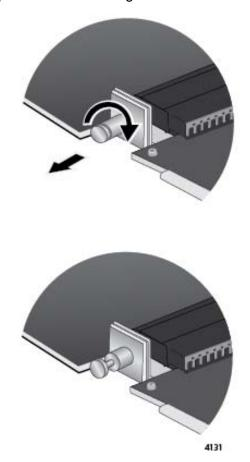
Figure 162. Retracting the Retaining Pin on the AT-SBx81XLEM Line Card
