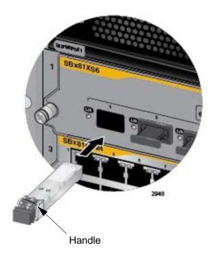
Figure 96. Installing an SFP+ Transceiver in the AT-SBx81XS6 Line Card
