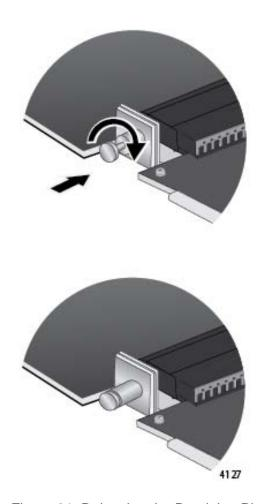
Figure 81. Releasing the Retaining Pin
