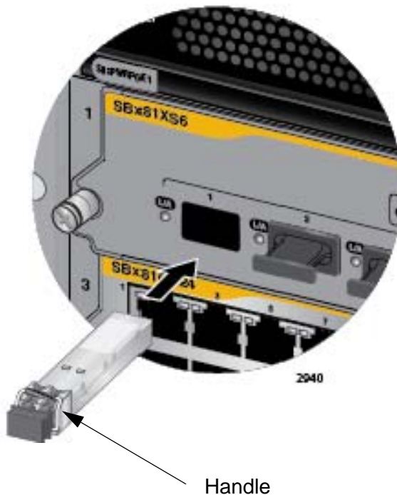
Figure 100. Installing an SFP+ Transceiver in the AT-SBx81XS6 Line Card
