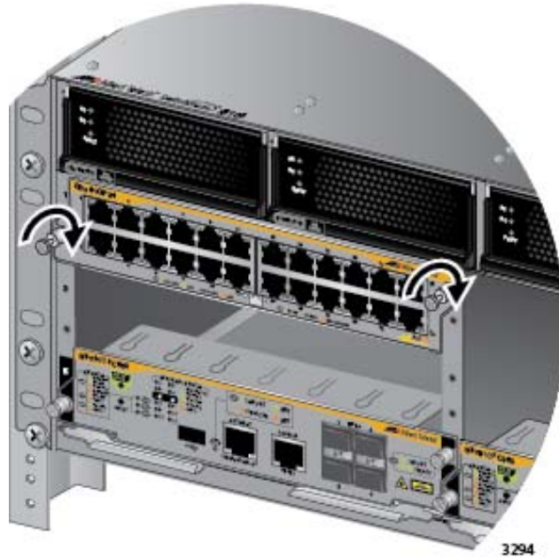
Figure 93. Tightening the Thumb Screws on an Ethernet Line Card
