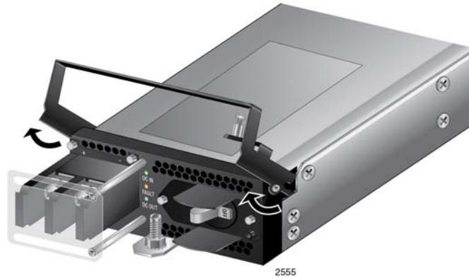
Figure 66. Raising Handle on the AT-SBxPWRSYS1 DC Power Supply
