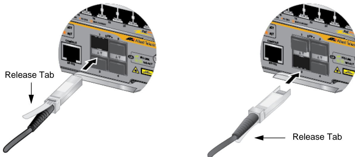
Figure 115. Installing an AT-SP10TW Cable in the AT-SBx81CFC960 Controller Fabric Card
