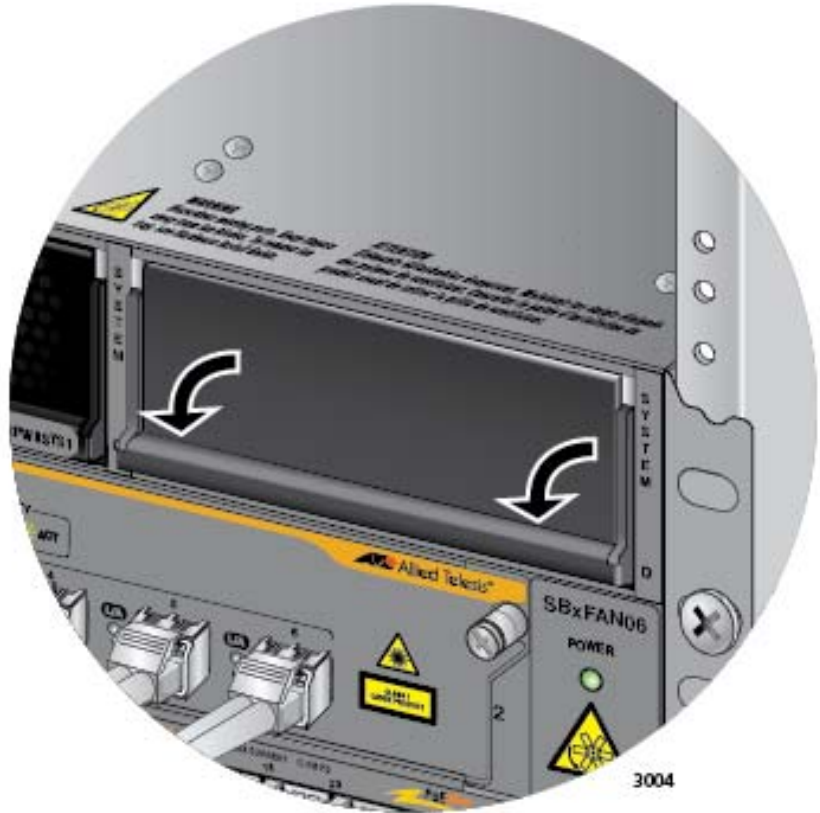
Figure 160. Lowering the Locking Handle on the Power Supply Slot Cover
