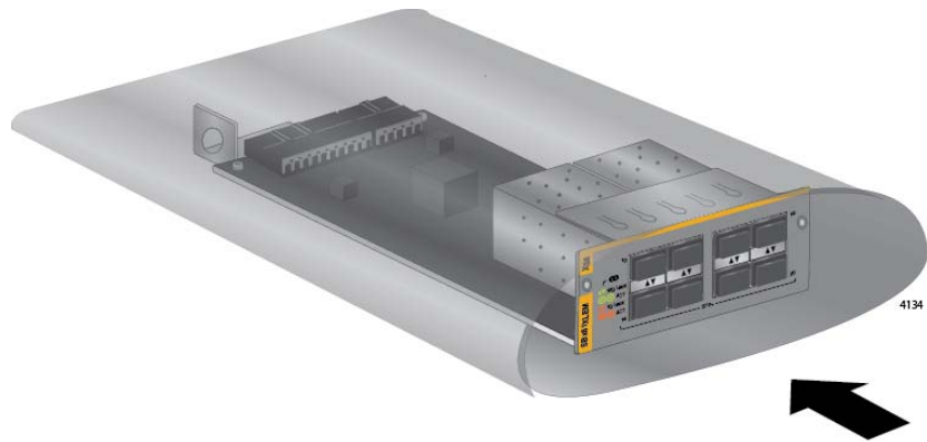
Figure 176. Storing the Expansion Module in an Anti-static Bag
