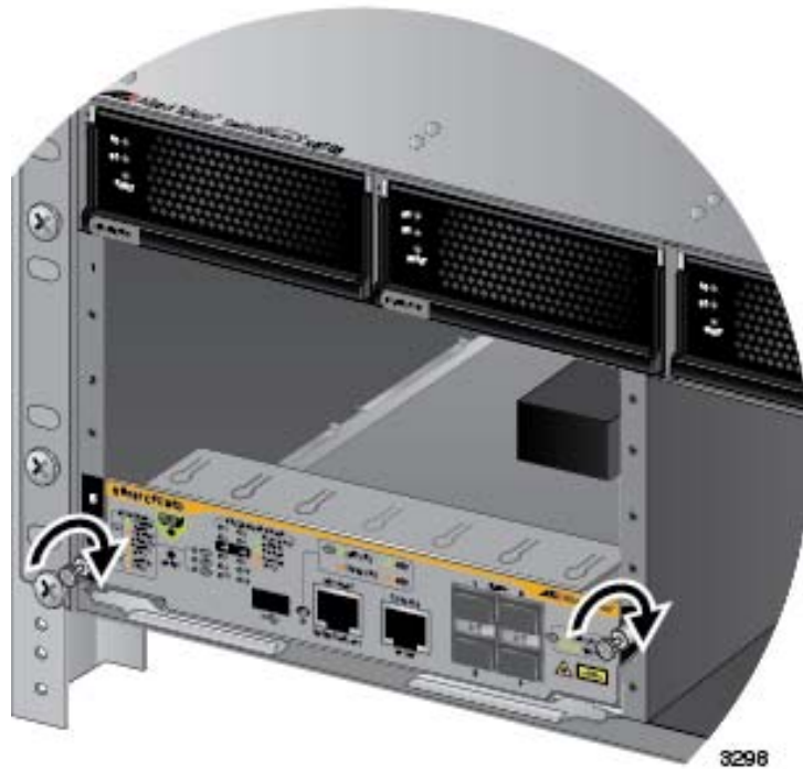
Figure 77. Tightening the Thumb Screws on the AT-SBx81CFC960 Card
