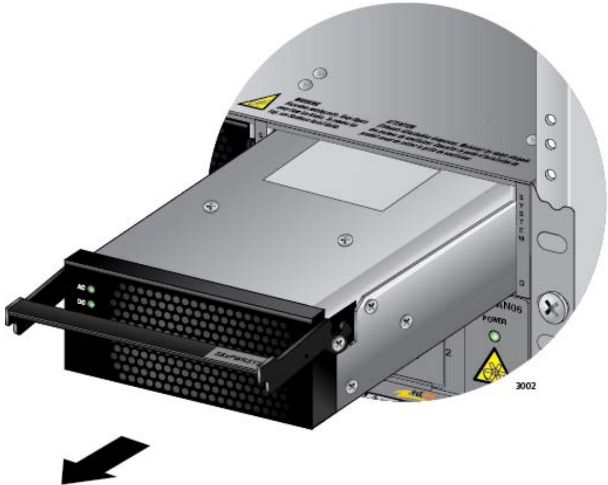
Figure 158. Removing the Power Supply from the Chassis
