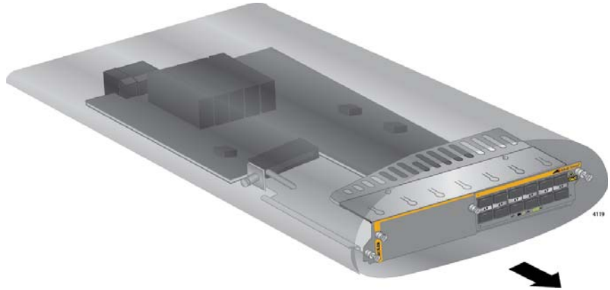
Figure 78. Removing the AT-SBx81XLEM Line Card from the Anti-static Bag
