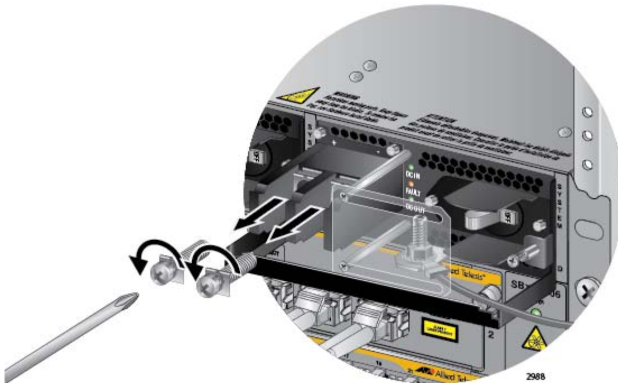
Figure 136. Removing the Terminal Screws
