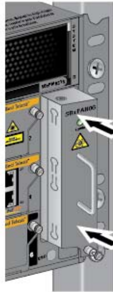
Figure 185. Securing the AT-SBxFAN06 Fan Module on the Backplane Connector
