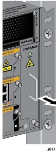
Figure 181. Loosening the AT-SBxFAN06 Fan Module from the Backplane Connector
