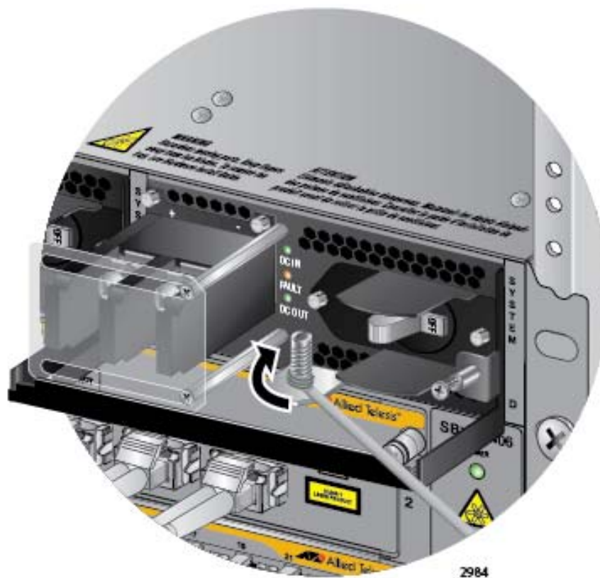
Figure 129. Attaching the Bare Grounding Wire to the Grounding Post
