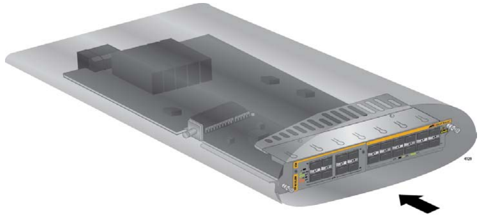
Figure 88. Returning the Line Card to its Anti-static Bag
