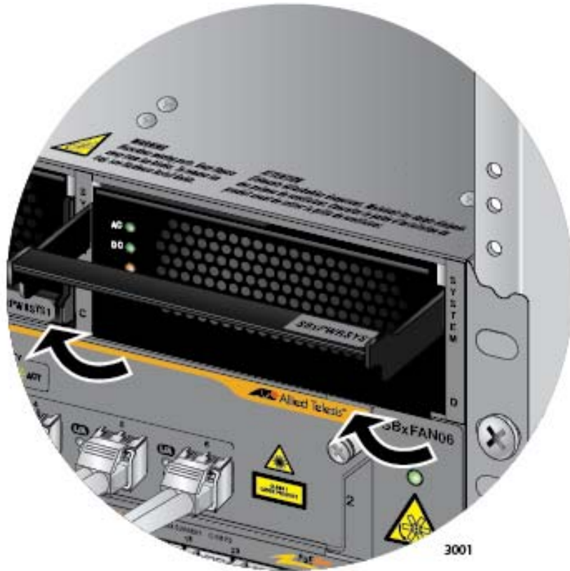
Figure 157. Lifting the Locking Handle on the Power Supply
