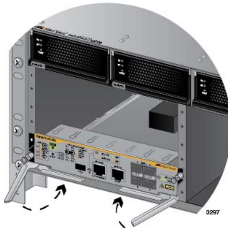
Figure 76. Closing the Locking Levers on the AT-SBx81CFC960 Controller Fabric Card
