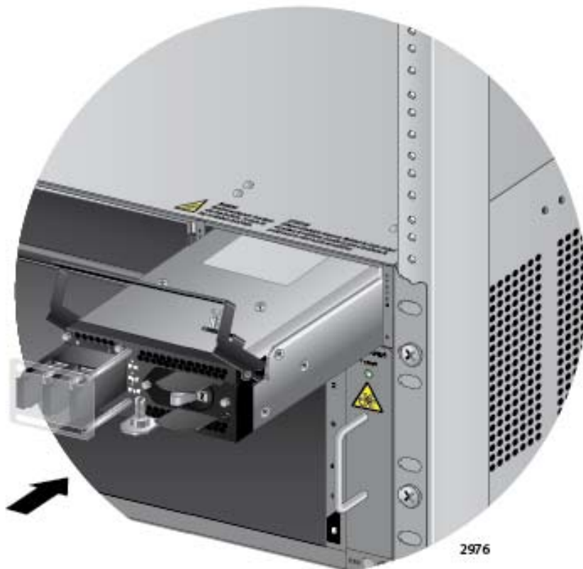
Figure 67. Inserting the AT-SBxPWRSYS1 DC System Power Supply
