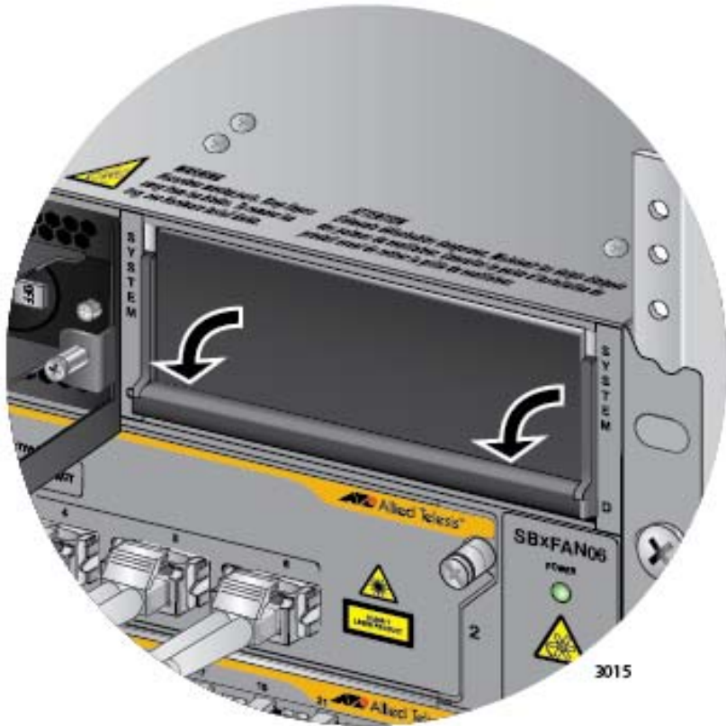
Figure 171. Lowering the Locking Handle on the Power Supply Slot Cover
