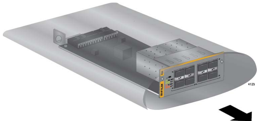
Figure 82. Removing the Expansion Module from the Anti-static Bag
