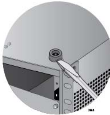
Figure 39. Removing the Rubber Feet
