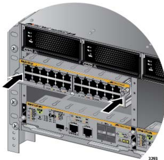
Figure 92. Seating an Ethernet Line Card on the Backplane Connector
