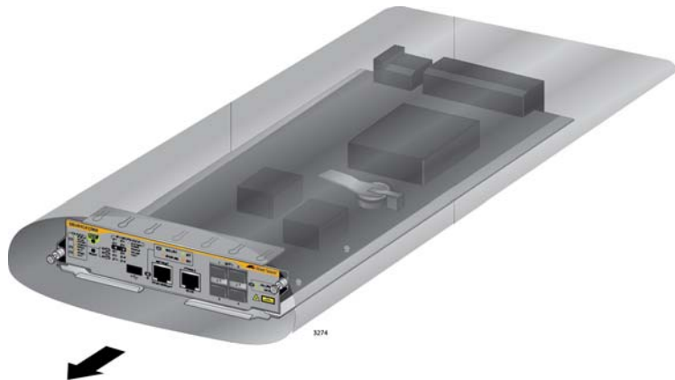
Figure 72. Removing the AT-SBx81CFC960 Controller Fabric Card from the Anti-static Bag
