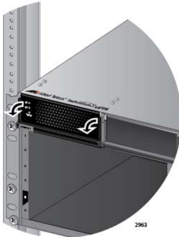
Figure 61. Locking the Handle on the AT-SBxPWRPOE1 Power Supply
