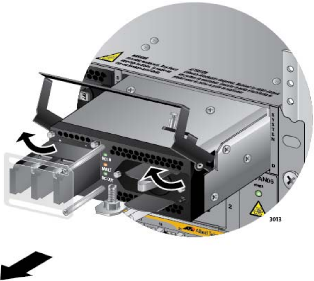
Figure 169. Lifting the Locking Handle and Removing the Power Supply
