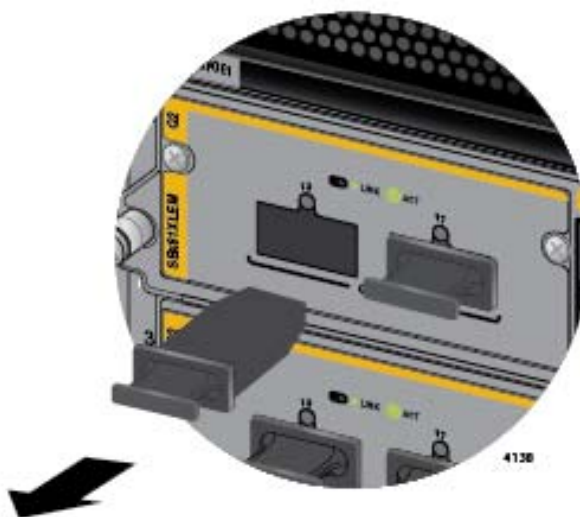
Figure 107. Removing the Dust Cover from a Slot on the AT-SBx81XLEM/Q2 Expansion Module
