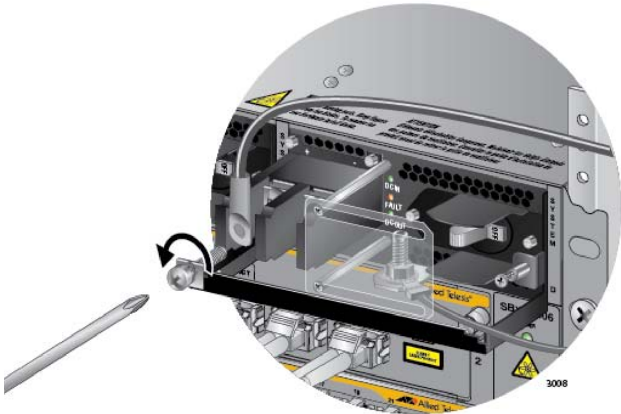
Figure 164. Removing the Positive Lead Wire from the Terminal Block
