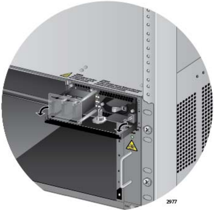
Figure 68. Locking the Handle on the AT-SBxPWRSYS1 DC System Power Supply
