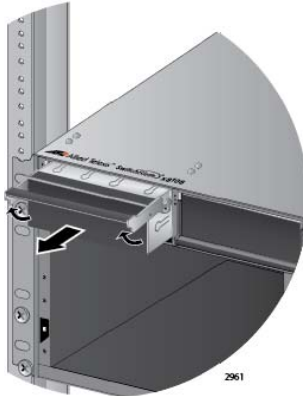
Figure 57. Removing the Blank Slot Cover from Power Supply Slot A
