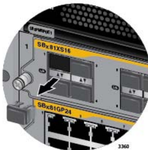
Figure 104. Removing the Dust Cover from an SFP+ Slot
