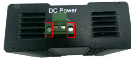
FIGURE 2-4 Securing Connector with Two Outside Screws
