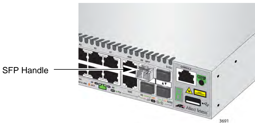
Figure 55. Positioning the SFP Handle in the Upright Position
