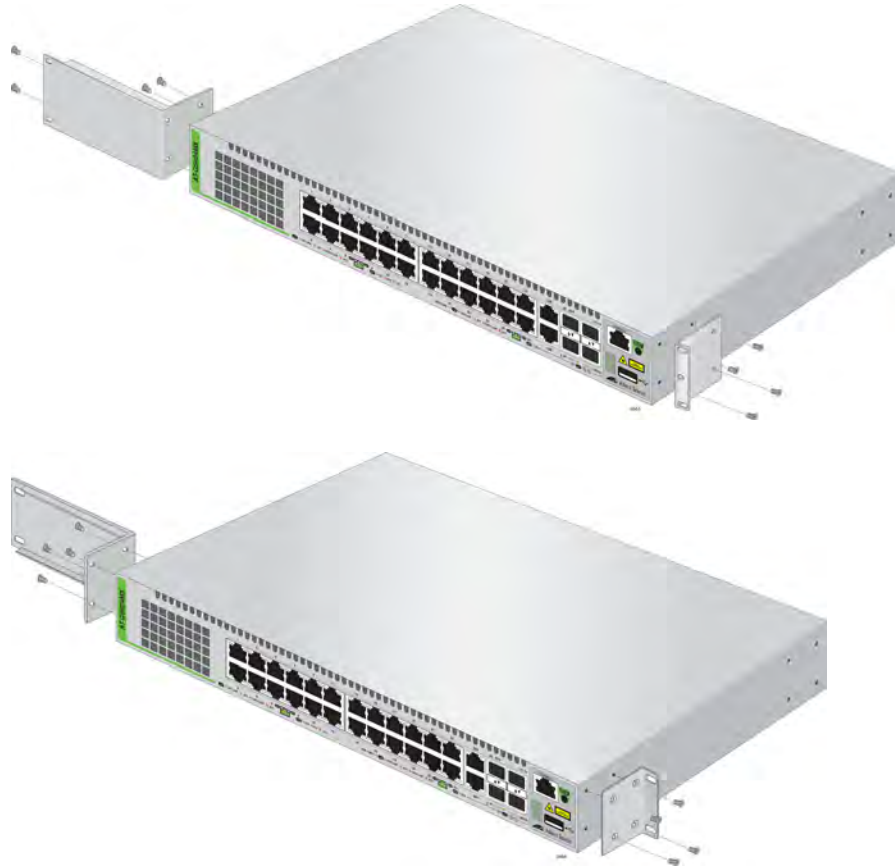
Figure 25. Installing Brackets on the AT-GS924MX Switch
