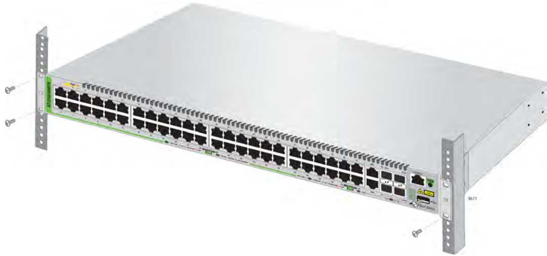
Figure 28. Mounting the Switch in an Equipment Rack
