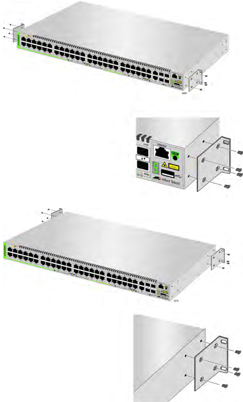
Figure 27. Attaching Brackets to the AT-GS924MPX, AT-GS948MX, or AT-GS948MPX Switch (Continued)
