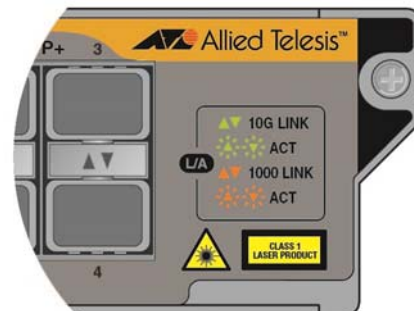
Figure 39. Legends for the SFP+ Ports on the AT-SBx81CFC960 Versions 1 and 2 Controller Cards
