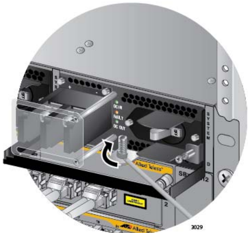
Figure 135. Attaching the Bare Grounding Wire to the Grounding Post
