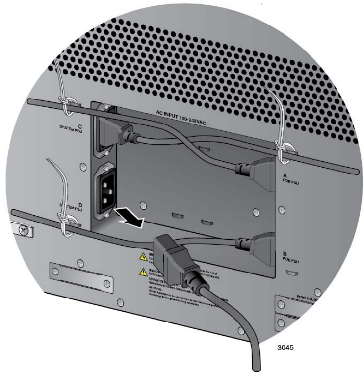
Figure 162. Disconnecting the AC Power Cord from the AC Socket on the Back Panel
