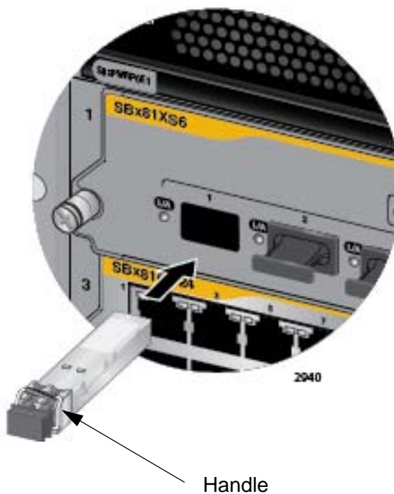
Figure 106. Installing an SFP+ Transceiver in the AT-SBx81XS6 Line Card
