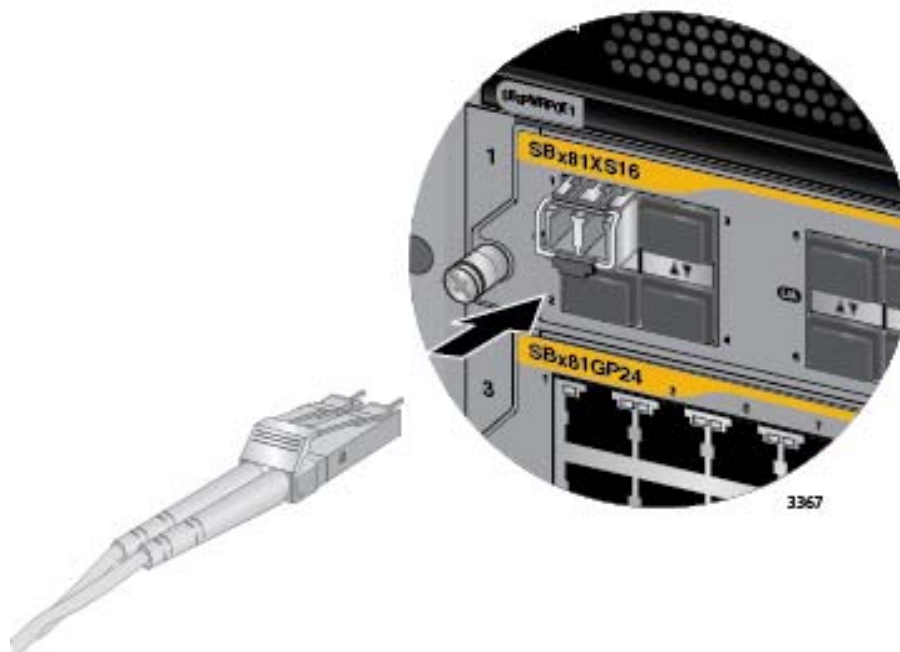
Figure 109. Attaching a Fiber Optic Cable to a Transceiver in the AT-SBx81XS16 Line Card
