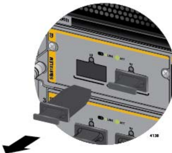
Figure 113. Removing the Dust Cover from a Slot on the AT-SBx81XLEM/Q2 Expansion Module
