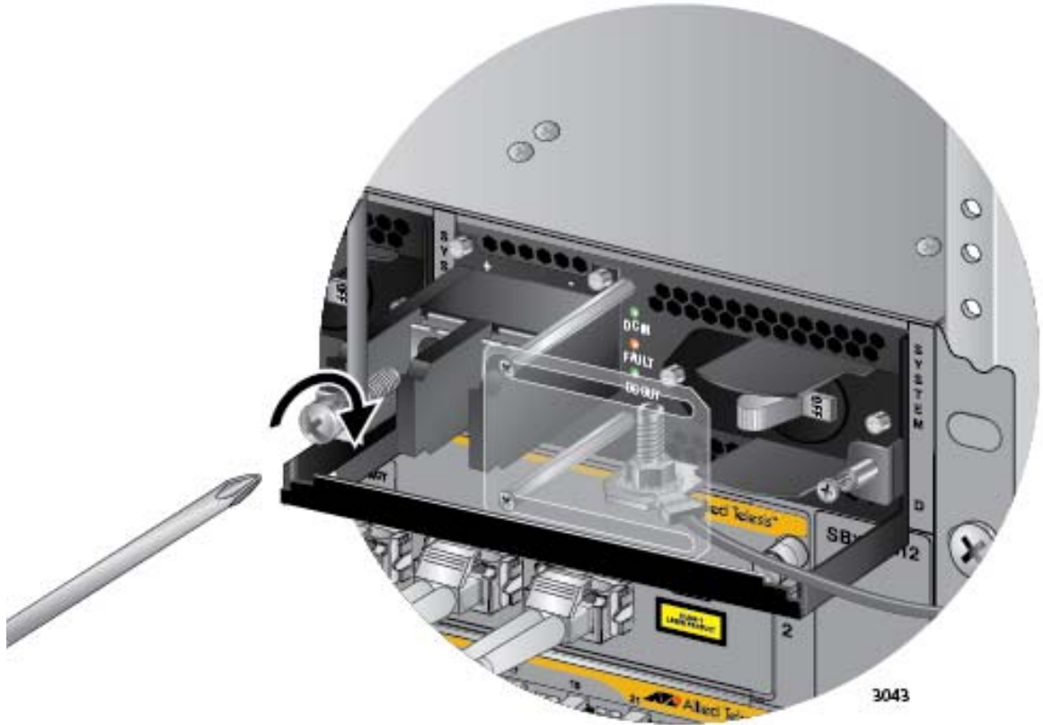
Figure 155. Connecting the Positive Wire With Bare Wire
