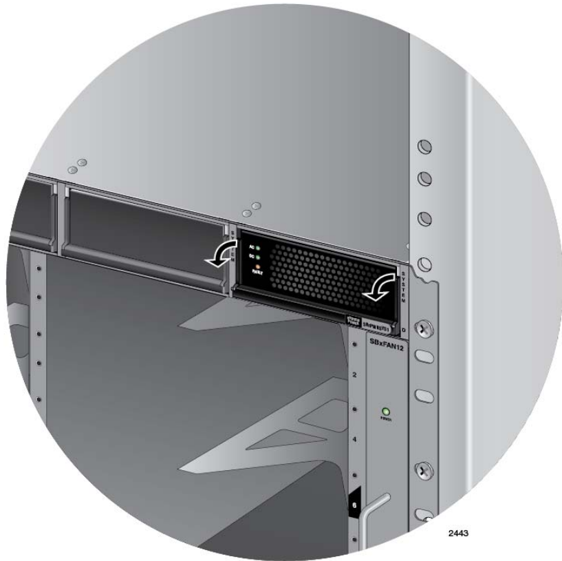
Figure 61. Lowering the Handle on the AT-SBxPWRSYS1 or AT-SBxPWRSYS2 AC System Power Supply
