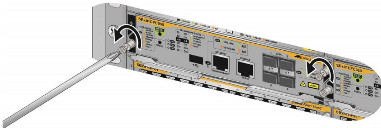
Figure 186. Loosening the Screws on the AT-SBx81CFC960 Controller Card
