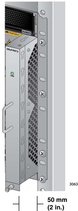
Figure 191. Withdrawing the AT-SBxFAN12 Fan Module 51 mm (2 In.) from the Chassis
