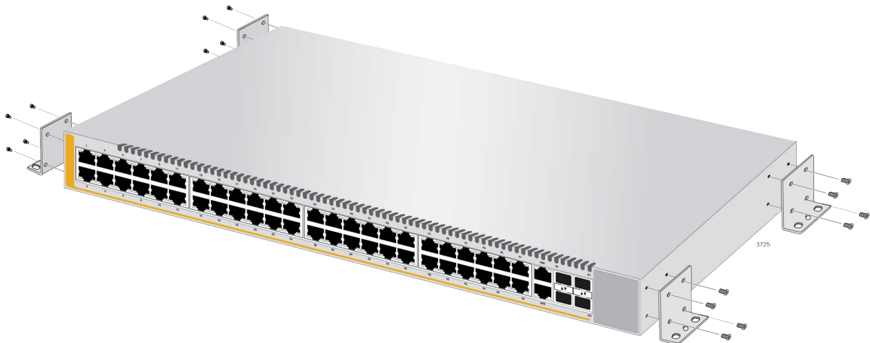
Figure 61. Installing the Brackets to the Switch for Wall Installation
