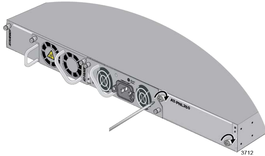
Figure 40. Tightening the Captive Screws on the Blank Panel for the Power Supply Slot
