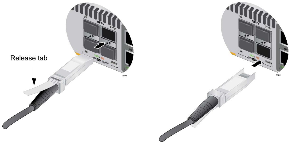
Figure 90. Installing AT-SP10TW Cables
