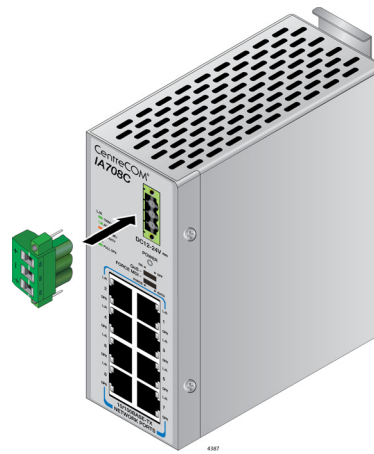
Figure 5. Attaching the 3-in Terminal Block
