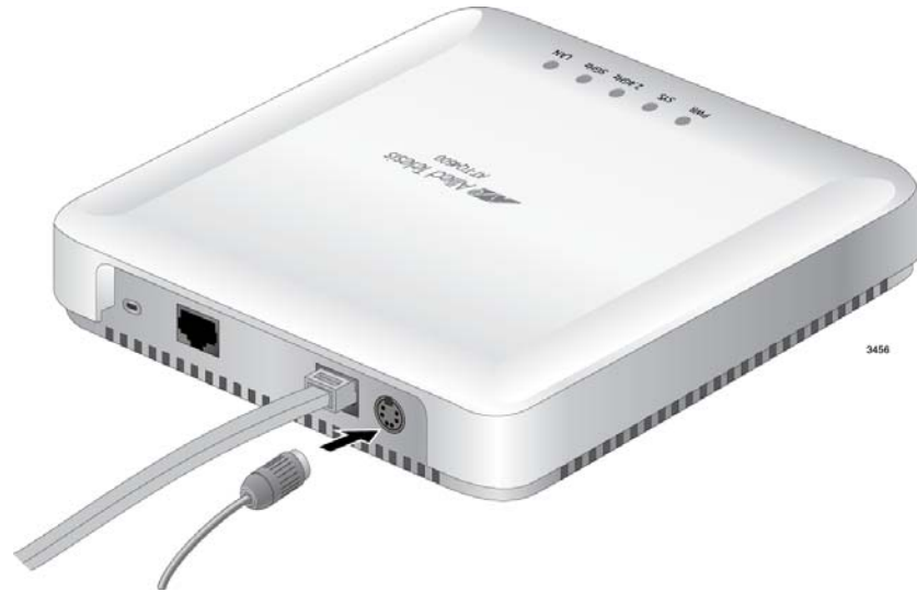
Figure 15. Connecting the Power Cable from the AT-TQ0091 AC/DC Adapter
