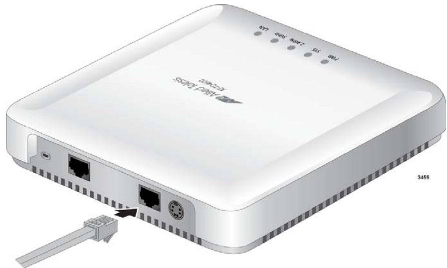
Figure 14. Connecting a Network Cable to the LAN Port
