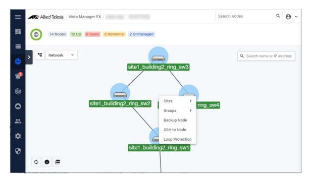
Loop protection is managed from the integrated map. You can select one or multiple (up to 10) devices from the integrated map for loop protection configuration. Once you have selected the devices that you want to configure, right click on one of them and select Loop Protection from the pop-up menu.
