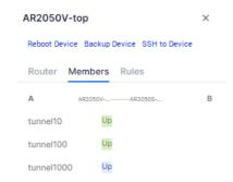
SD-WAN rules associated with this router. The colours here represent the status of each tunnel as described above.
