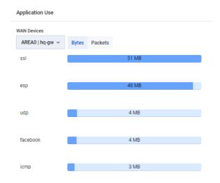
The application use chart shows the amount of data sent and received for a device, broken down by application. You can select which device to view from the WAN Devices drop-down. You can also choose whether to view bytes or packets by choosing the appropriate toggle.
