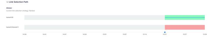
The Link Selection Path chart shows a time-line of which link is being used for the selected rule. You can see which link selection strategy is being used, and the history of which link has been chosen.
