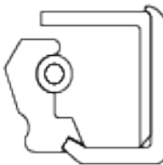
SB Profile Oil Seal 5 PSI - Single Lip
