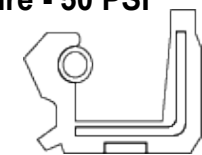
SA / C Profile Oil Seal 5 PSI - Single Lip
