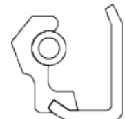
SC / A Profile Oil Seal 7 PSI - Single Lip
