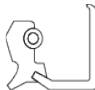
TC / AS - Profile Oil Seal - 7 PSI BABSL - Medium Pressure - 50 PSI Double Lip
