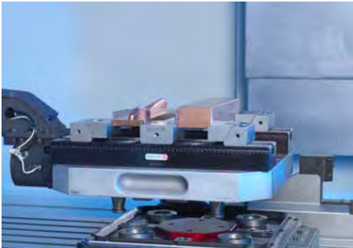
The part feeding system with pallet handling is perfectly suited for medium-sized batches and single parts. Various clamping devices may be mounted on the pallets without having to program a robot.
