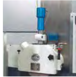
Automatic linear diamond device "Bermi" on head
