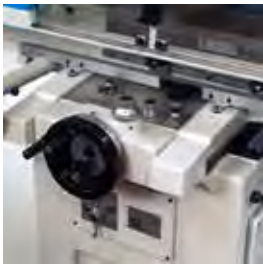
Cross slide with 0.001 release
