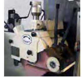
Upsetting tool for "Bermi" grinding wheels with 2 slides
