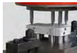
Rotary riveting station to secure the terminals on a capacitor using two radial riveting machines RN 081
