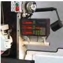
Display "Bermi Control" with 2 or 3 axes
