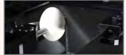
vice for thin-walled workpieces this clamping system can even clamp an egg!
