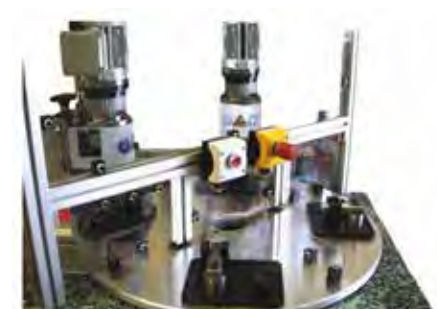
Rotary riveting station to secure the terminals on a capacitor using two radial riveting machines RN 081
