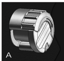
View A shows knob in 'rest' position. View B shows the top section retracted to allow entry of padlock shackle
