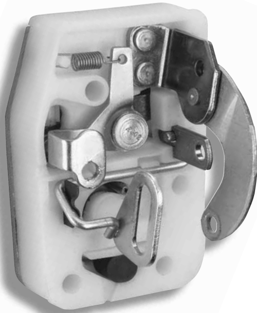
9/02142 Right side latch showing operating levers
