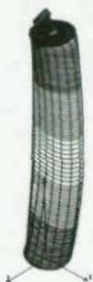
Figure 2a. Four Node Thin Shell Element Model Showing Exaggerated Deflection Patterns Under a Radial Live Load Along its Length
