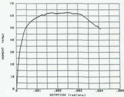
FIGURE 10 MOMENT-ROTATION CURVE FOR SECTION 152x152x23
