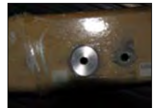
Hole prepared by the new ATI Burnishing Kit using the type 'N' pads demonstrating an absolute perfect surface for overall contact.
