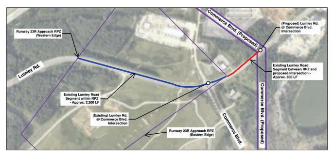
Figure 2: Approximate length of Lumley Road within RPZ and prior to proposed intersection
