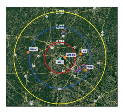
An initial cost analysis was performed for each quarry in which a production rate of 24,000 CY of borrow material per day, which matches the estimated rate of the proposed conveyor system, was held constant for an even comparison. As the distance from RDU increases more than a few miles, this assumed production rate becomes unrealistic as the number of trucks necessary to meet this rate becomes impractical.
