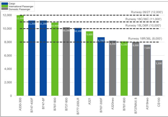
Notes: A330-900neo manufacturer planning data is not available. The A330-300 was used as a viable substitute in the runway length analysis.
