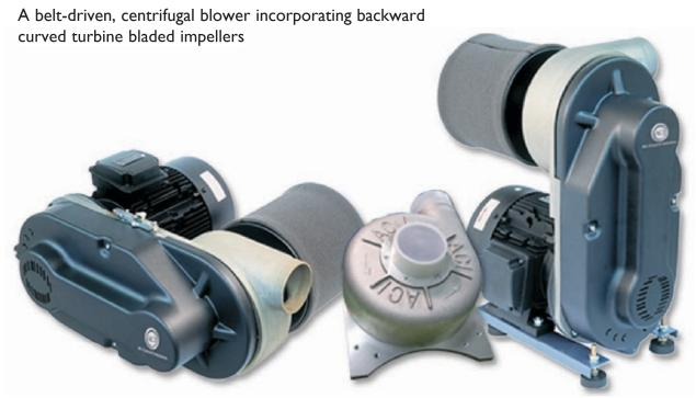
Powerful and robust, ACI's EP10A Compact Blowers incoporates a backward curved turbine bladed impeller. They are available with motors from 5.5 through to 18.5kW in standard metric or NEMA frames and can be easily retrofitted in place of other belt driven alternatives. Due to its relatively small footprint, the EP10A is ideal for integrating into customer's equipment.
