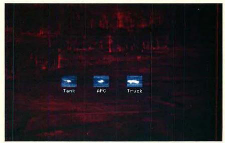
Infrared systems will deliver a wealth of information to pilots and Weapon System Officers. This sensor, in tandem with the Hughes's Electro-Optical Signal Processing Computer, not only shows the raw images, it also automatically differentiates the various target types. It is not out of the question that systems of the future will be able to detect heat from even so small a target as an individual enemy soldier.
