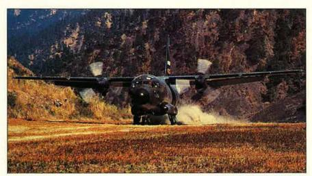
The C-27A intratheater airlifter for Southern Command will be a modified version of the Aeritalia G.222 STOL transport (here, coming in for a landing on a dirt strip). The C-27s will fill the airlift gap between CH-47s and C-130s in Central America.
