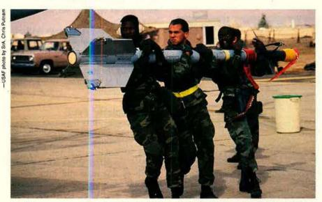
Munitions crew members from the 33d TFW load a Sidewinder onto an F-15, just one of the many types of munitions available to Desert Storm pilots. Crew members were nonchalant about keeping up with the astonishing 2,000 combat sorties per day. "It's like a 7-Eleven," said one. "The pilots can get any bomb they like."
