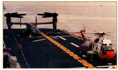
The number four V-22 Osprey flight test aircraft prepares for takeoff from the deck of USS Wasp (LHD-1). The V-22's wing has been rotated into position, and the rotor blades are about to be unfolded. Completion of initial shipboard compatibility trials last December was an important milestone in the aircraft's development.
