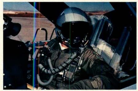
The Combat Edge G-suit ensemble reduces fatigue and almost doubles the time a pilot can withstand high-G forces. The ensemble uses two oxygen hoses, one to the pilot's mask (and the bladder that keeps the mask sealed tightly to his face) and one to the counterpressure garment (the vest under the harness straps).
