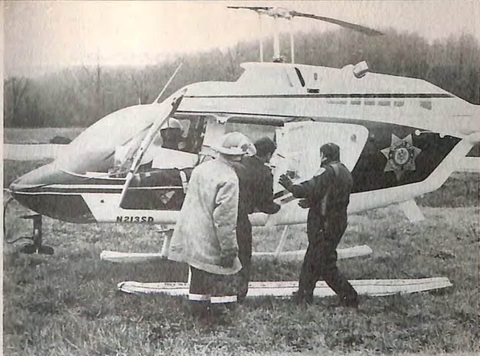
In New York State, the Onondaga County Sherrif Department's Bell 206B III helicopter is equipped to handle medical evacuations.
