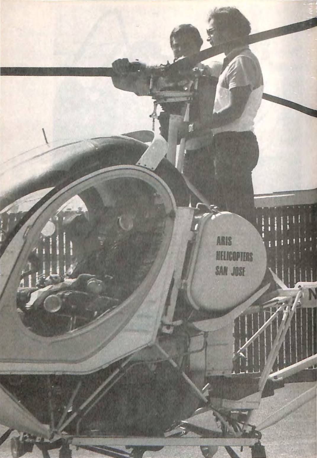
In San Jose, CA., an Aris Helicopter's flight instructor and student do a pre-flight inspection of the main rotor.
