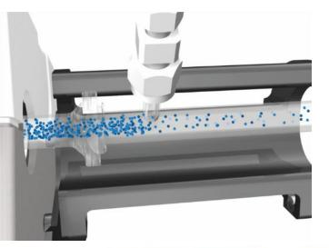
HMI is an aerosol dilution technique It dilutes the sample using a make-up flow of argon gas, added after the spray chamber Increases matrix tolerance 10x
