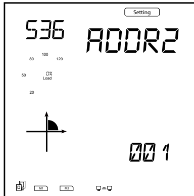
Figure 5-53 Address Setting for AXM-RS485
