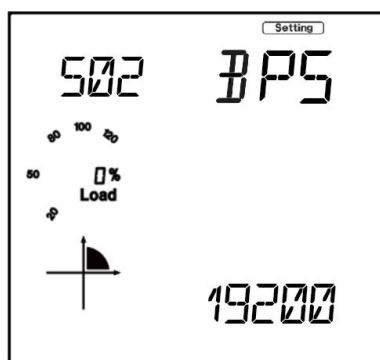
Figure 6-3 System Parameter Setting - S02 Baud Rate
