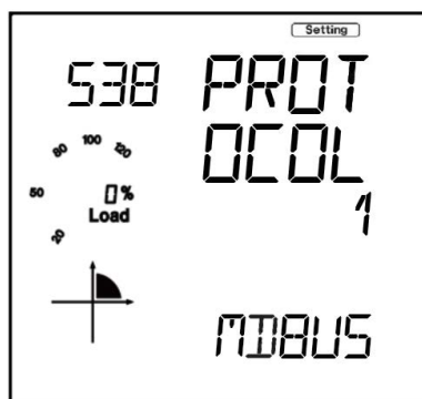
Figure 6-4 System Parameter Setting - S38 Protocol 1
