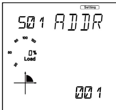
Figure 6-2 System Parameter Setting - S01 Address
