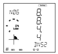
Press 'P' to get to "N07 Modbus Port". Press 'V/A' to configure the Modbus Port. The cursor of
