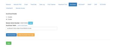
**NOTE:** The "TEST AcuCloud" button should only be utilized after clicking the 'Save' button otherwise a failure response will be observed. If a failed response occurs after clicking 'Save', please double check the serial number entered in AcuCloud, the token entered in the web page as well as viewing the test post details by clicking on the 'Details' option.
