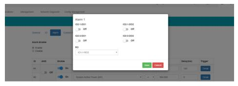
Once all alarm settings are configured, user must click on the 'Save' button and then reboot the communications module for the settings to take effect.
