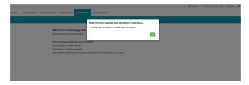
After the meter reboots, users will be able to log back into the web interface. When logged in, click on the 'About' navigation tab located on the top right corner of the web page to view the 'Device Information' page. Users can check this page to confirm the meter's firmware version was updated correctly.
