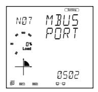
• Press 'P' to get to "N08 HTTP Port". Press 'V/A' to configure the HTTP Port. The cursor of the first digit will begin to flash. Press the 'H' button to scroll through the digits, press the 'P' or 'E' to change the value of the flashing cursor and press 'V/A' to confirm.
