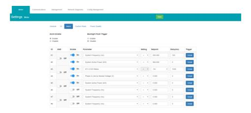
If extended I/O modules are being used, users can click on the detail tab to configure the digital output and relay outputs to be triggered when an alarm is triggered.
