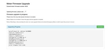
When the firmware update is complete, the module will reboot. The rebooting process will take 1 to 2 minutes to complete.
