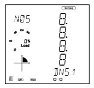
• Press 'P' to get to "N06 DNS Secondary Server". Press 'V/A' to configure the DNS address. The cursor of the first digit will begin to flash. Press the 'H' button to scroll through the digits, press the 'P' or 'E' to change the value of the flashing cursor and press 'V/A' to confirm.
