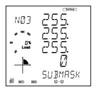
• Press 'P' to get to "N04 Gateway". Press 'V/A' to configure the gateway IP address. The cursor of the first digit will begin to flash. Press the 'H' button to scroll through the digits, press the 'P' or 'E' to change the value of the flashing cursor and press 'V/A' to confirm.
