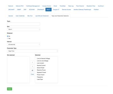
Once configured, on you can verify on your MQTT server if the data is being received. The data is received in ISON format.
