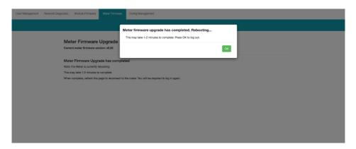
Log into the web interface of the AXM-WEB2 series module after the reboot is complete and go to the 'About' page to check if the module firmware version is updated.
