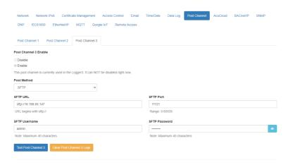
Click the 'Save' button after changing any settings. Users will be prompted to reboot the AXM-WEB2 series module immediately or at a later time. If later is chosen the AXM-WEB2 series module must be rebooted from the 'Management' page for the settings to take effect.
