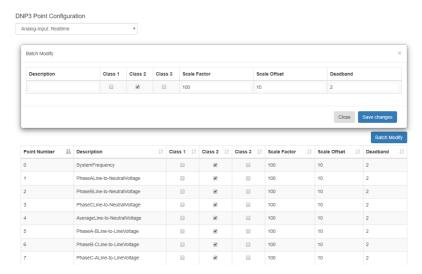
After all DNP settings are complete, click on the 'Save' button. Users will be prompted to reboot the AXM-WEB2 series immediately or at a later time. If later is chosen the AXM-WEB2 series must be rebooted from the 'Management' page for the settings to take effect.
