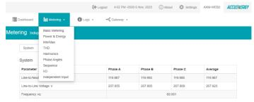
When enabling the independent channel feature, the independent input will appear in the drop-down menu under metering. Users can view the corresponding values:
