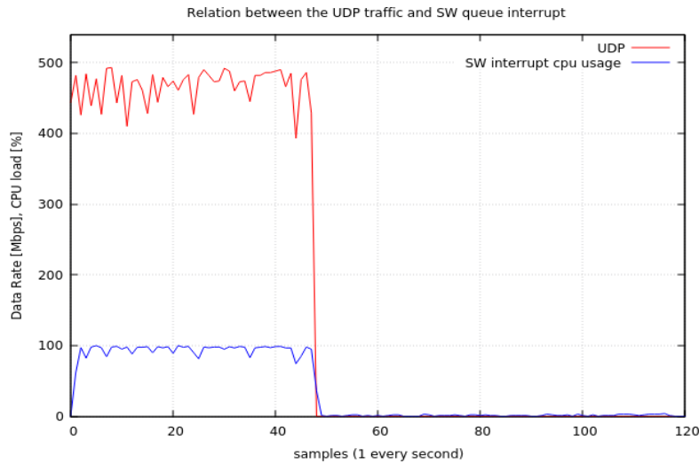
Figure 2-27: UDP throughput degradation due to high queuing interrupt activity that overload the CPU capacity.
