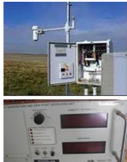
Figure 6-11: AN/FMQ-8 Temperature Dew Point Measurement Set, sensor and electronics on top and indicator on bottom.
