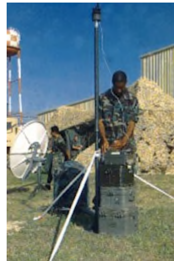
Figure 7-3: A1C Eric Andrews takes an observation with the TMQ-34 Tactical Meteorological System.
