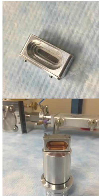
The picture above shows the primary, secondary and tertiary layers. The picture below, show the holder in the protective layer, and screwed to the paddle
