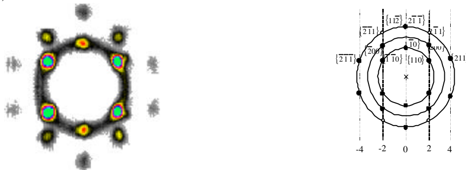
Figure 2. Scattering map for a Tetronic 908 (4 branches star polyPOE co POP) solution at 30% in D 2 O (T = 47°C) oriented by a shear rate \dot{\gamma} = 371 \text{ s}^{-1} (left hand side) compared with theoretical figures for body centered cubic lattice.
