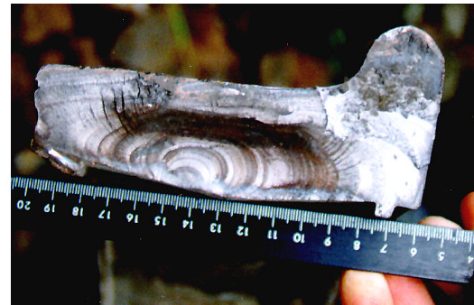
Figure 4. Fracture surface of a broken railway wheel hoop.
