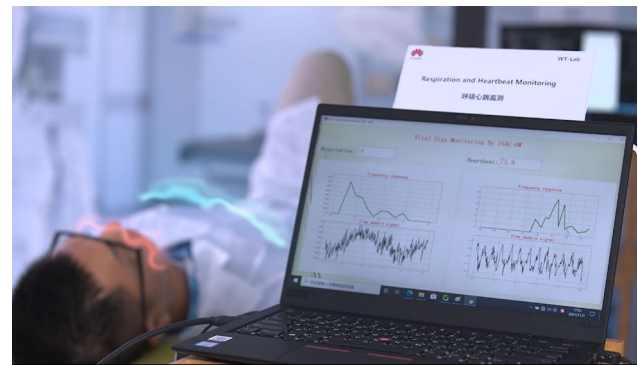
Figure 7 Remote health monitoring: ISAC prototype
