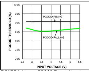
FIGURE 2-14: PGOOD Threshold vs. Input Voltage.
