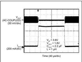
**FIGURE 2-23:** Load Transient (50 mA to 750 mA).
