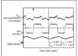
FIGURE 2-21: Switching Waveform Continuous Mode (500 mA).
