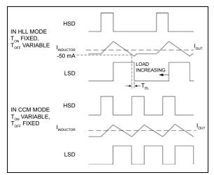
**FIGURE 5-1:** HSD Signals for t<sub>ON</sub> Control, Inductor Current and LSD for t<sub>OFF</sub> Control.
