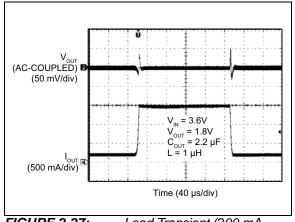
**FIGURE 2-27:** Load Transient (200 mA to 1.5A).
