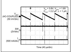
**FIGURE 2-19:** Switching Waveform Discontinuous Mode (1 mA).
