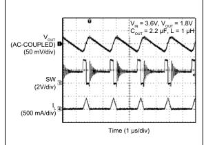
*FIGURE 2-20:* Switching Waveform Discontinuous Mode (50 mA).
