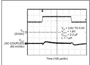
**FIGURE 2-28:** Line Transient (3.6V to 5.5V @ 1.5A).
