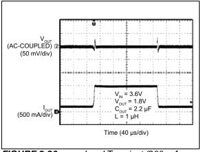
**FIGURE 2-26:** Load Transient (200 mA to 1.5A).
