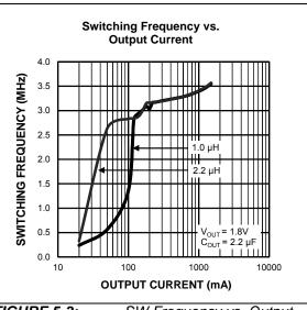
FIGURE 5-3: SW Frequency vs. Output Current.
