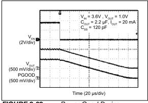
FIGURE 2-32: Power Good During Shutdown.
