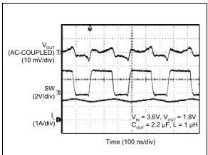
FIGURE 2-22: Switching Waveform Continuous Mode (1.5A).
