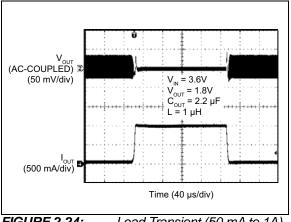
FIGURE 2-24: Load Transient (50 mA to 1A).
