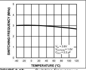
FIGURE 2-17: Switching Frequency vs. Temperature.
