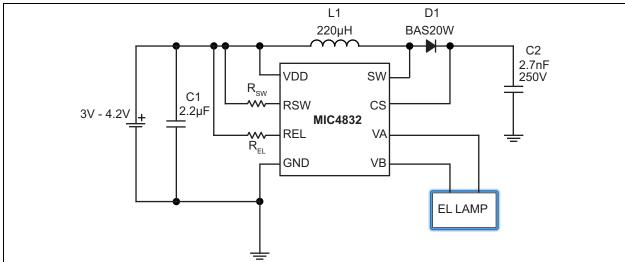
FIGURE 6-1: Typical Li-lon Powered MIC4832 Circuit.
