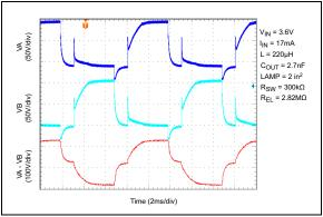
FIGURE 4-1: 100 Hz Output Waveform
