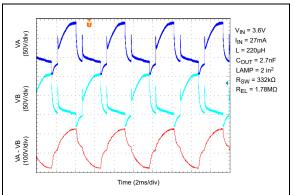
FIGURE 4-2: 200 Hz Output Waveform.
