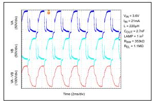
FIGURE 4-3: 300 Hz Output Waveform.
