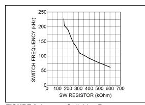
FIGURE 2-1: SW Resistor.
