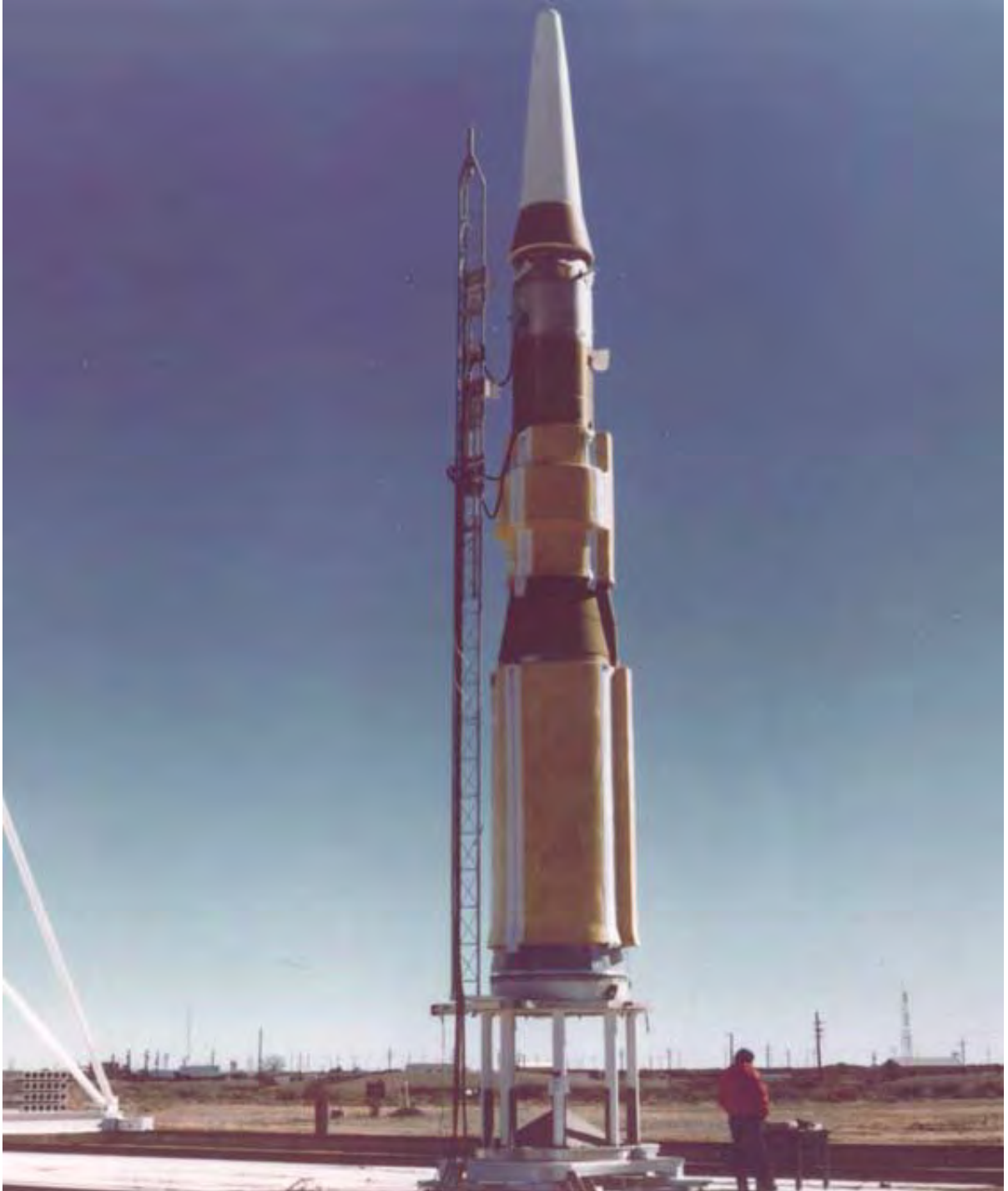
Figure 54. A Hera Target Missile on its launcher pedestal at LC-32 ( adapted from Walker et al. 2003 ).
