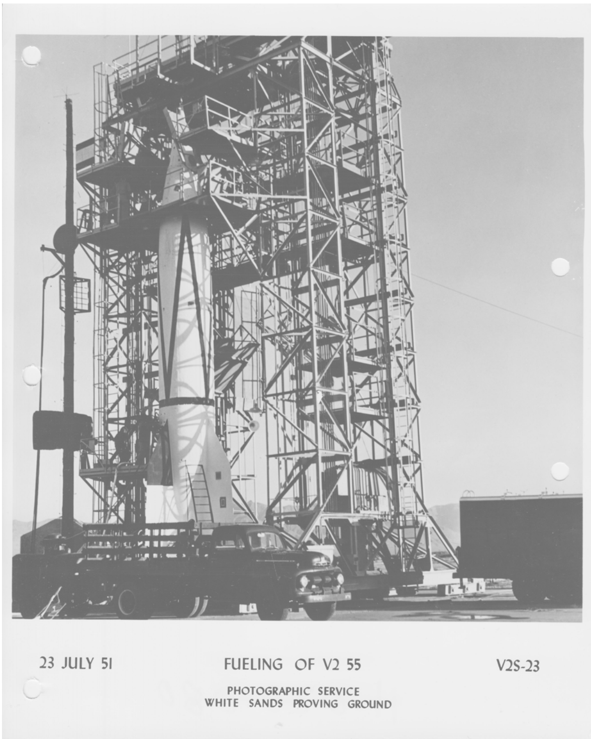
Figure 16. A V-2 on the gantry at LC-33 in 1951 ( courtesy WSMR Museum Archives ).
