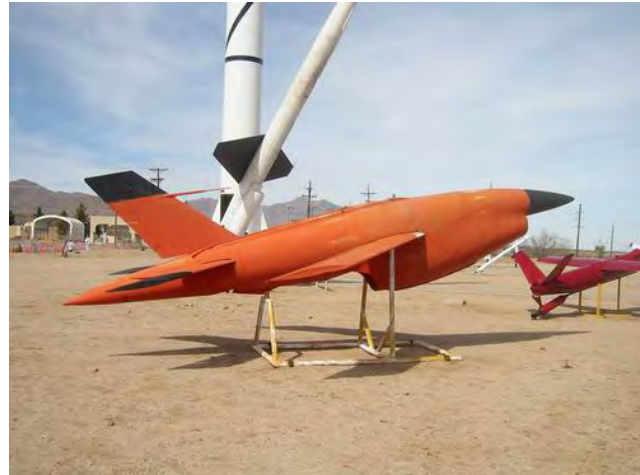
Figure 49. The improved Firebee Q-2C configuration with its “chin” intake location ( photo courtesy WSMR Museum ).
