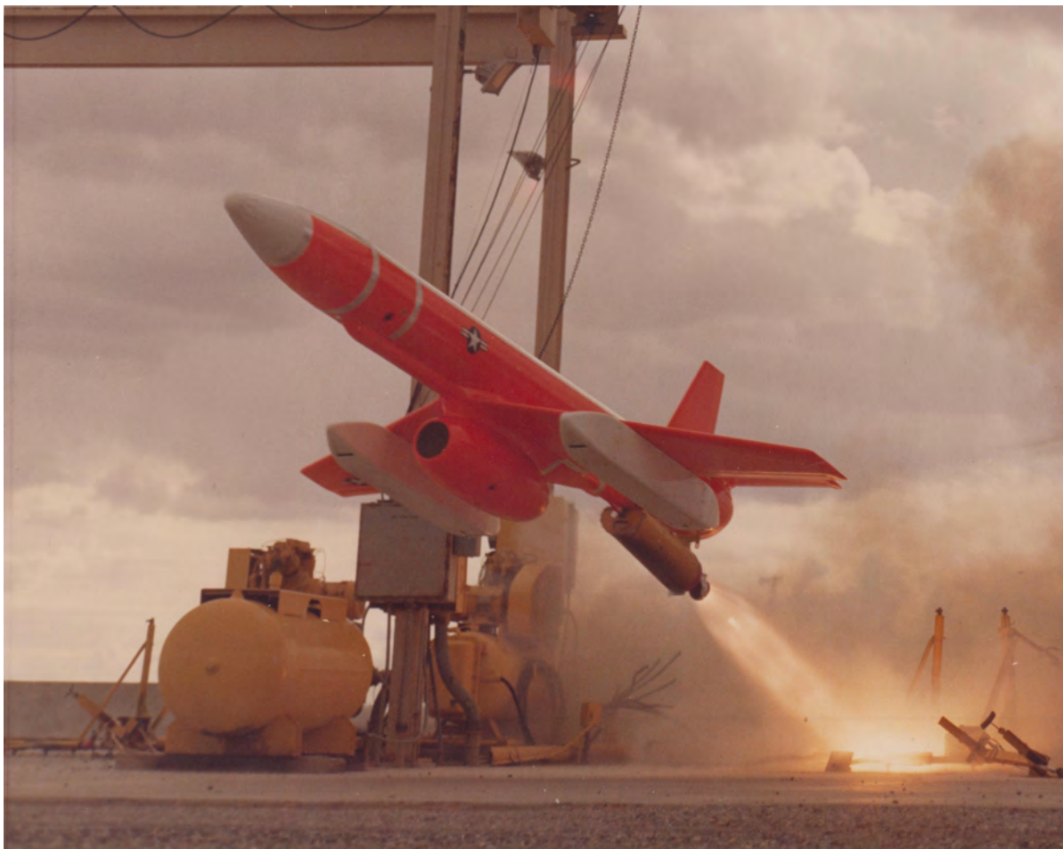
Figure 50. A MQM-107 Streaker drone launch at the LC-32 MTLC in 1983. Note the JATO booster (courtesy WSMR Museum Archives).
