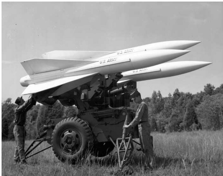
Figure 31. Basic Hawk missiles on mobile launcher trailer, circa early 1960s ( courtesy Redstone Arsenal ).
