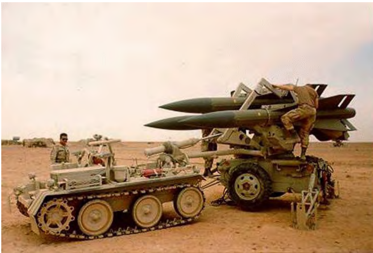
Figure 35. Loading an I-Hawk launcher trailer using the M501 loader vehicle, circa early 1990s (courtesy Federation of American Scientists).
