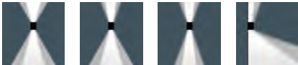
[M/M] Medium beam, up and down [E/M] Narrow beam up, medium beam down [E/E] Narrow beam, up and down [E/A60] Narrow beam up and 'forward throw' down
