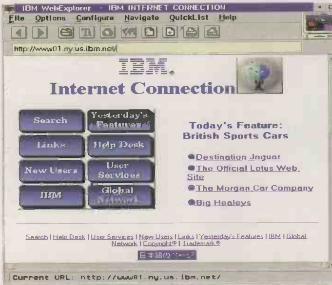
Fig. 3. The IBM home page at http://www01.ny.us.ibm.net . This page is intuitive in use yet downloads quickly due to careful design. It works well with or without graphics, which in total amount to only 12Kbytes.
