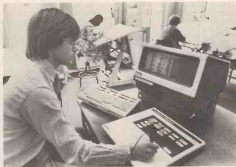
The instrument being used here is the Redac "Cadet" p.c.b. designer, the complete system having been launched recently by Racal-Redac. It is a microprocessor-based system which the makers say is the first true example of computer-aided design in this field and at a "reasonable" price. This particular system costs £20,000.
