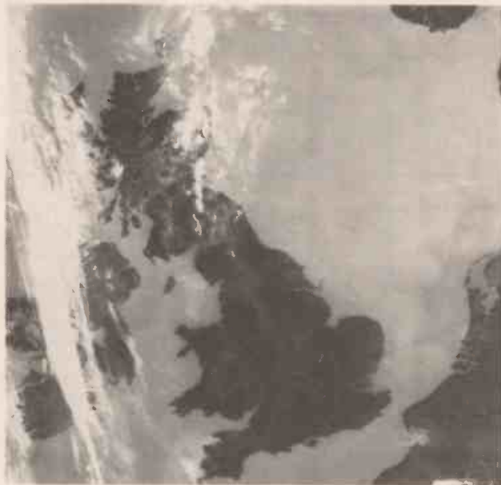
A high definition heat study of the British Isles taken by satellite, NOAA-6, equipped with infra-red sensors, from an altitude of 833km. The darker land mass denotes the relatively warmer ground temperatures compared with the sea —
