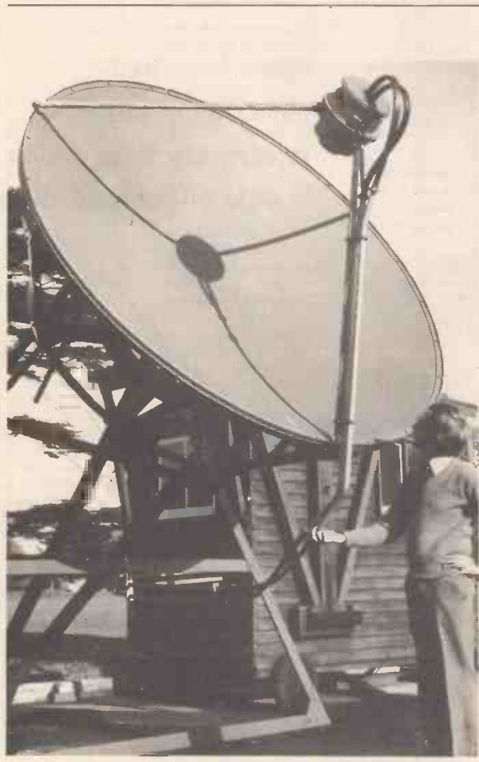
A 2.4 metre dish used by BBC engineers to receive experimental signals from OTS. The BBC hopes to be able to take up two of the five channels allocated for satellite broadcasting in Britain, one for pay television and the other to provide selected "best" programmes from BBC1 and BBC2.
