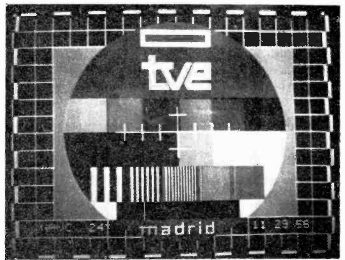
Spain RTVE (B, G) — Electronic test card which includes a digital clock. RTVE are experimenting with PAL colour.
