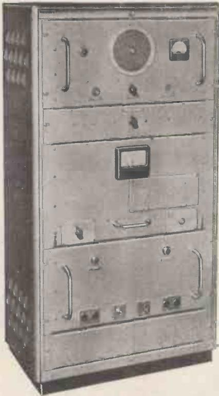
The new Pye 50 watt V.H.F. FIXED STATION is of an advanced design employing the latest techniques. It is ideal for use in normal fixed and mobile schemes where high powered transmitters are required and may also be used for point-to-point radio-telephone links.
