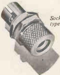
The connectors illustrated are designed for use with the smaller diameter R.F. cables, such as Telcon PT.1.M, PT.11.M, AS.60.M, etc. Produced for instrument designers and general application, the 58 Series Plug and Socket has a capacitance of less than 7  $\mu$ F. The 58C panel mounting socket shown will accept any plug in the 58P Series.
